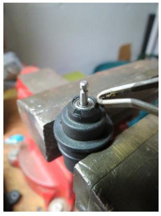
Insert the circuit board square with the end of the housing. Note that there is a locating boss opposite the three plastic clips. Using both of the pliers on opposite sides of the circuit board, squeeze lightly and evenly so the circuit board is pushed straight into the housing. The completion of this task can be done with your fingernails.
