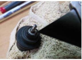
Next, using the needlenose pliers, grasp the plastic barrel that holds the four small magnets on the inside of the housing. Pull straight out. This is a press -fit on the shaft, no glue.
