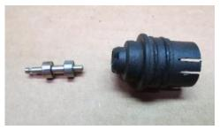
The shaft will probably have some dirt/debris/rust on the surface, so I chucked up the shaft using the middle area where the bearings don't ride using my battery drill. Holding the emery cloth or super fine sandpaper I cleaned both ends of the shaft.
