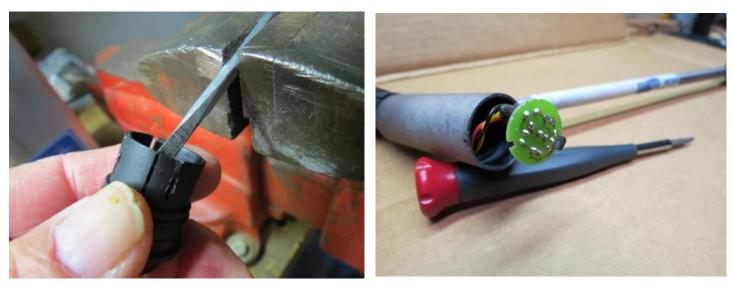
This left picture above shows the clamped screwdriver in place to push on the tab. For clarity I took this picture after I had removed the circuit board.
