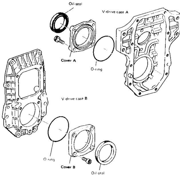
9-7 Insert the V-drive shaft into the V-drive case A, and insert the V-drive gear into the output shaft.
