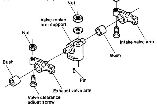
The same part is used for both intake valve rocker arm and exhaust valve rocker arm. The bush is not fitted to the valve rocker arm.
