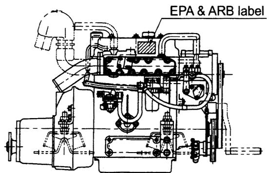
**\*3GM30F(C)(V):** attached to the top of the fresh water cooler.
