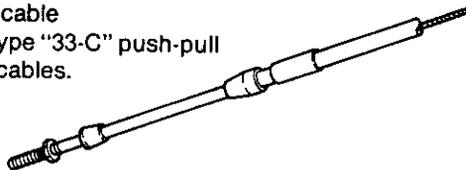
Use only Super-Responsive Morse Control Cables. They are designed specifically for use with Morse control heads. This engineered system of Morse cables, control head and engine connection kits ensures dependable, smooth operation with an absolute minimum of backlash. The thread size on cable ends is 10-32. Travel is up to 3". The core is a solid wire, with a 3/32" diameter.
