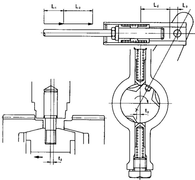
the holder is moved by the spring reaction so that the shift lever is pushed forward.
