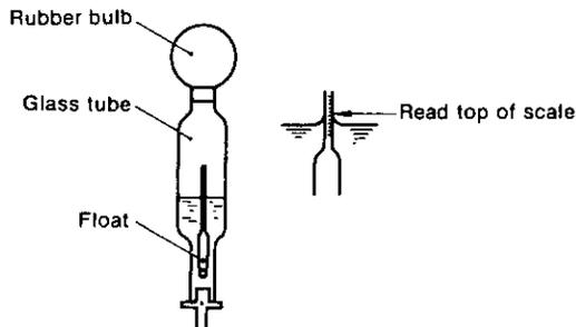
3) The battery is fully charged if the specific gravity is 1.260 at an electrolyte temperature of 20°C. The battery is discharged if the specific gravity is 1.200
