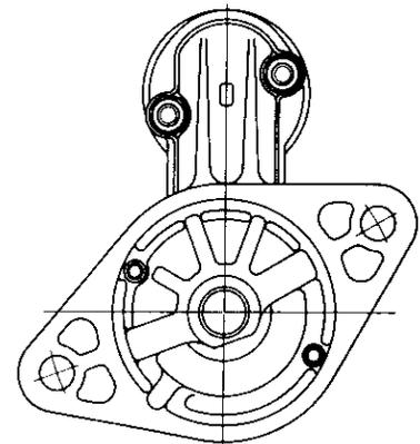
To prevent the motor receiving a shock which will occur as the engine starts and over-runs, this starter motor is installed with an over-running clutch.
