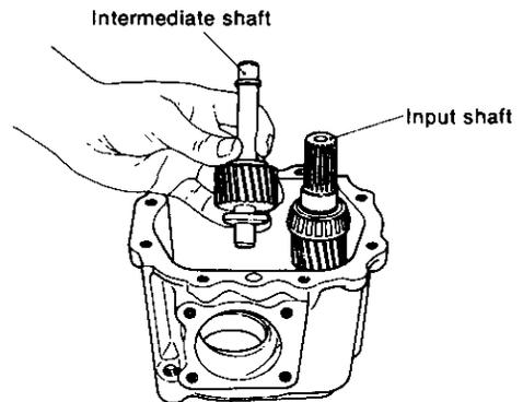
**NOTES:** 1) If the output shaft is not fitted into the clutch case before driving-in the intermediate shaft, it cannot be assembled.
