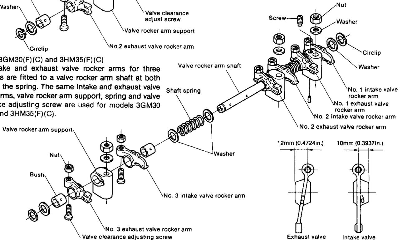
**2-6.2 Measuring the valve rocker arm shaft and bushing clearance**
