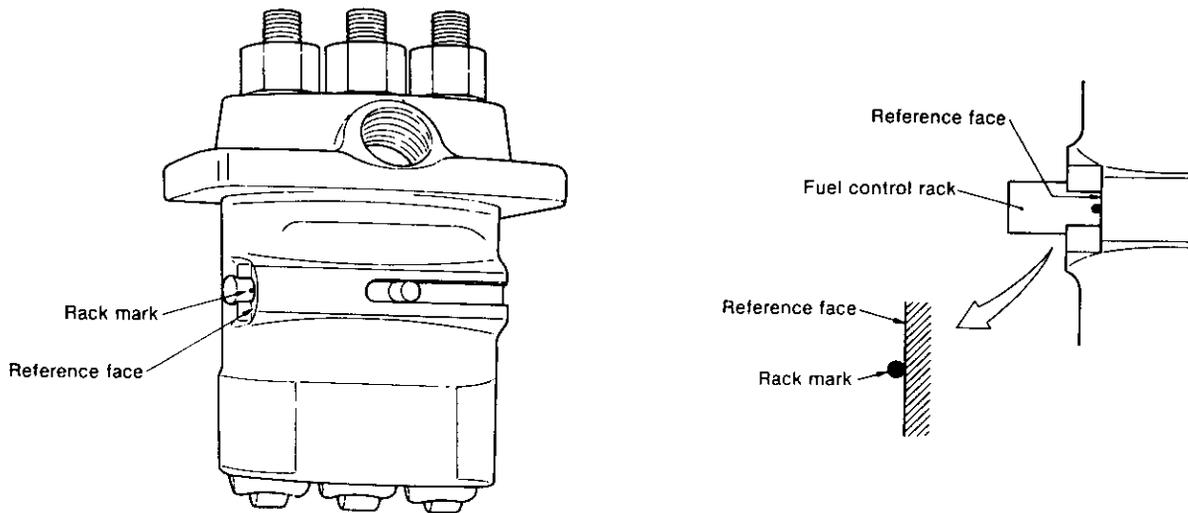
**NOTE:** When the engine is stopped, the control rack will automatically stay at the position which allows the maximum fuel injection volume. Therefore, to match the rack mark, move the engine stop lever to the position where the mark is matched and fix the lever at that position, then adjust so that the fuel limiter comes into contact with the lever.
