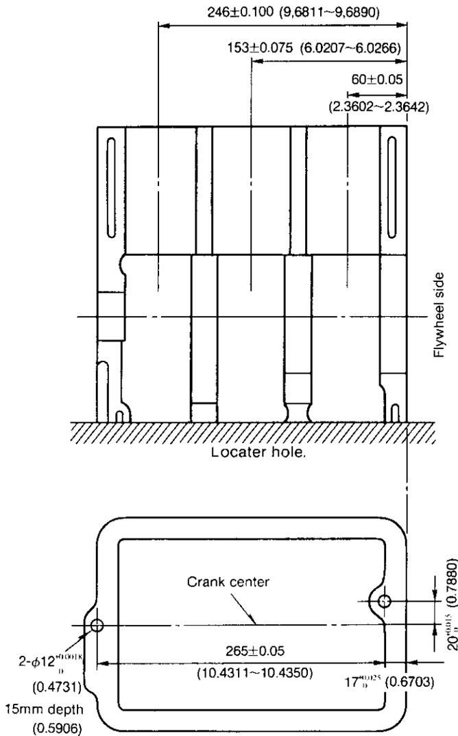
(1) How to measure distortion on the upper surface of the cylinder
