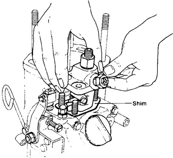
**CAUTION:** Note the number and total thickness of the timing adjustment shims.
