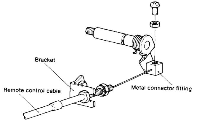
The metal connector fitting has a hole of 2.5mm (0.0984 in.) dia. to accommodate the cable, and cable of 1.5  $\sim$  2.5mm (0.05906  $\sim$  0.0984 in.) dia. can be used in the connector.
