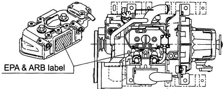
**\*3GM30(C)(V):** attached to the exhaust side of the rocker arm cover.
