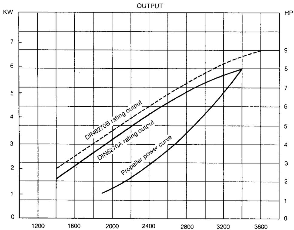
SPEED OF CRANKSHAFT: rpm
