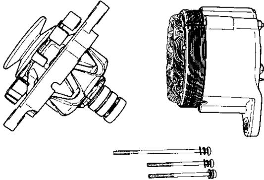
(2) Remove the pulley nut, and pull out the rotor from the front cover.
