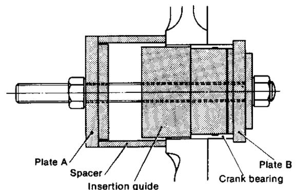
until it touches the cylinder block or bearing housing, using the puller/extractor as a guide, as shown in the figure.
