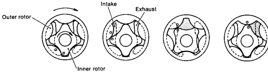
The lubricating oil pump is installed on the cylinder body at the timing gear case end, and its rotor shaft gear is driven by the crankshaft gear. The lubricating oil is drawn in and discharged through drilled holes in the cylinder body.
