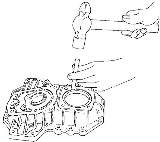
8-15 Remove the bearing inner races from the V-drive gear shaft.
