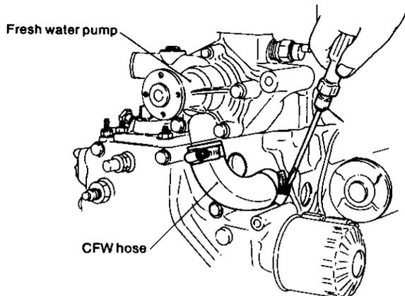
(2) Connect the CFW hose between the CFW pump and heat exchanger by connecting it to the CFW pump; tighten the hose clamp slightly. The hose clamp will be securely tightened after the heat exchanger is assembled.
