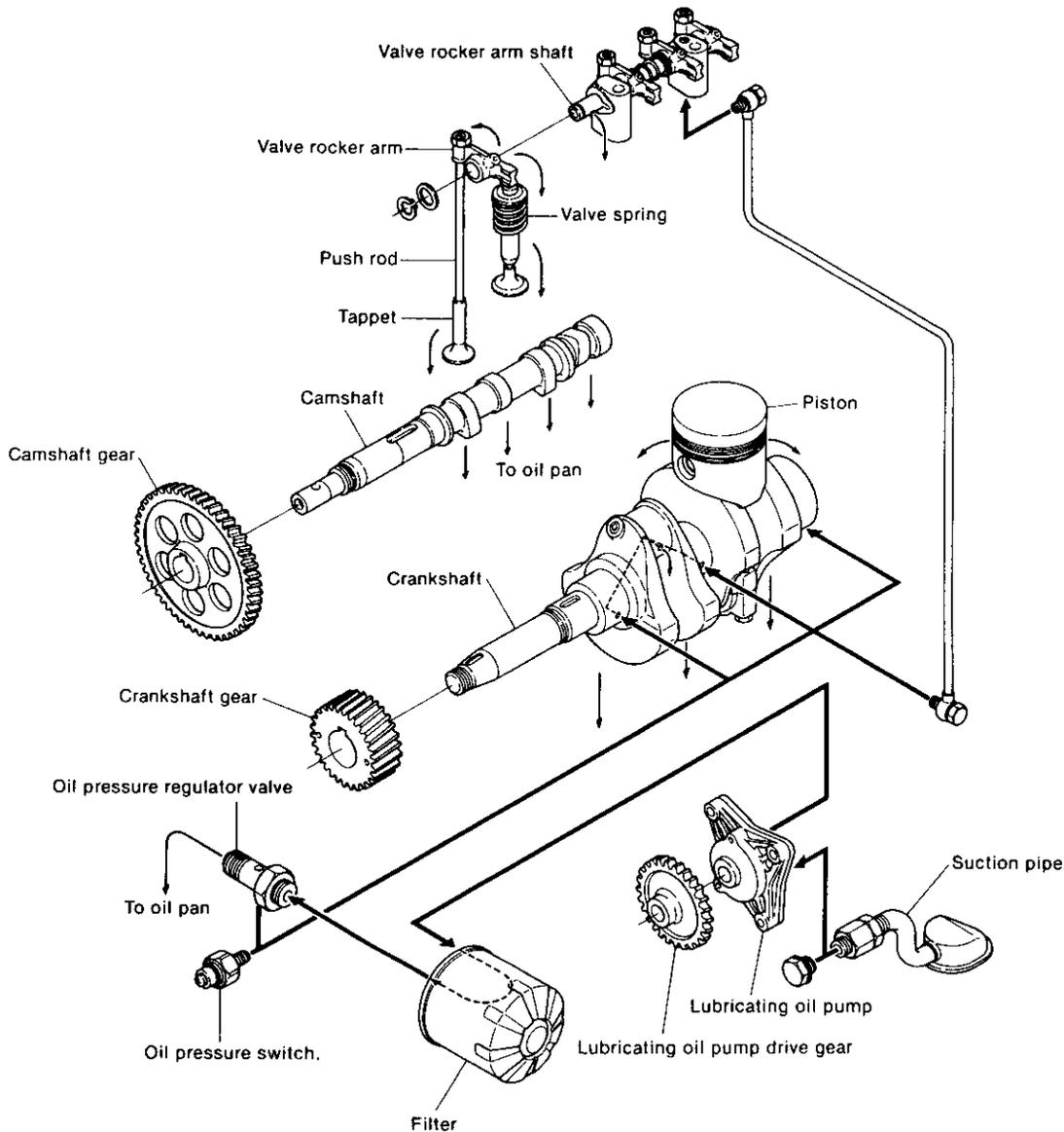
1-3 Lubrication oil passage of model 3GM30(F)(C) and 3HM35(F)(C)
