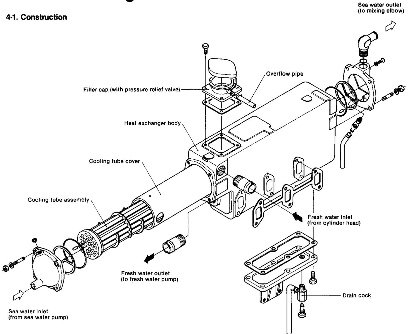
The heat exchanger uses sea water to cool the fresh water, which has reached a high temperature, while being circulated in the cylinder block.
