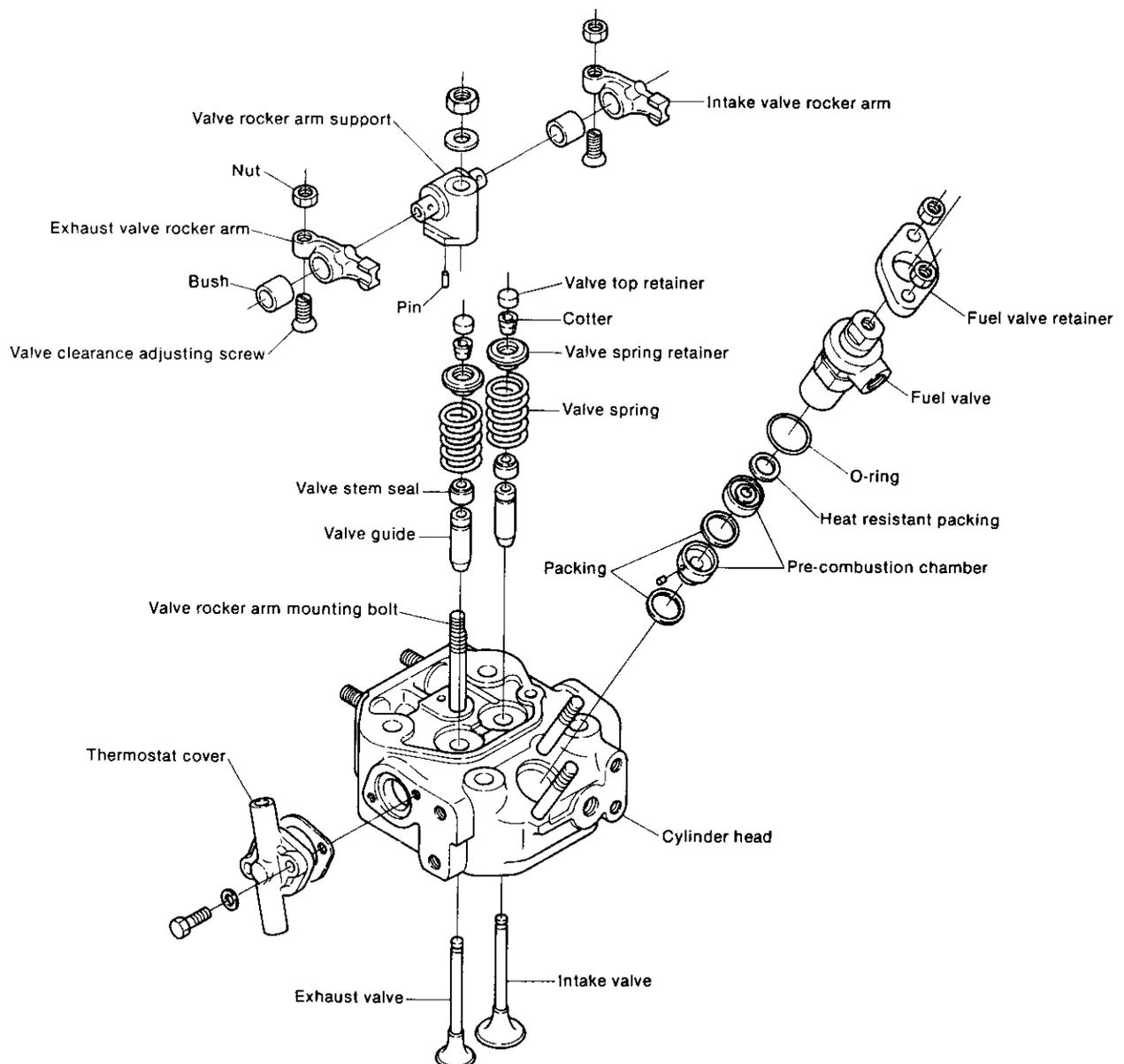
2-1.2 Cylinder head of model 2GM20(F)(C) engine
