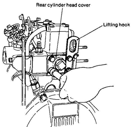
**2-17. Remove the fuel high pressure pipe**
