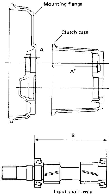
(2) Shim thickness (T2, T3) measurement of output shaft
