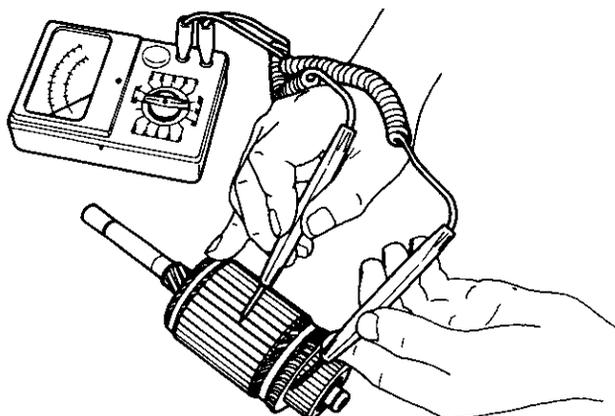
Checking armature windings for insulation faults.
