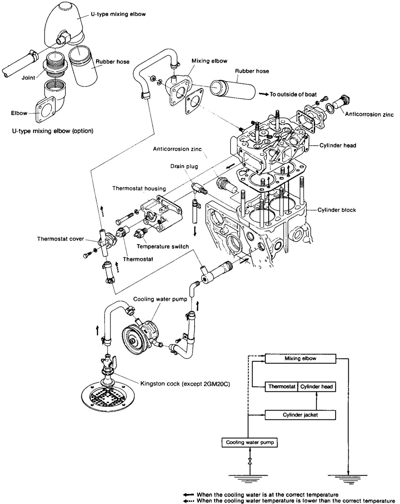
1-2.3 Cooling water passage of engine models 3GM30(C) and 3HM35(C)
