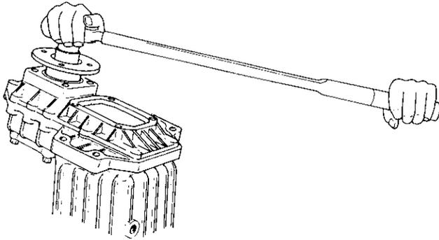
NOTE: 1) Use the special tool to remove the end nut from the V-drive shaft.
