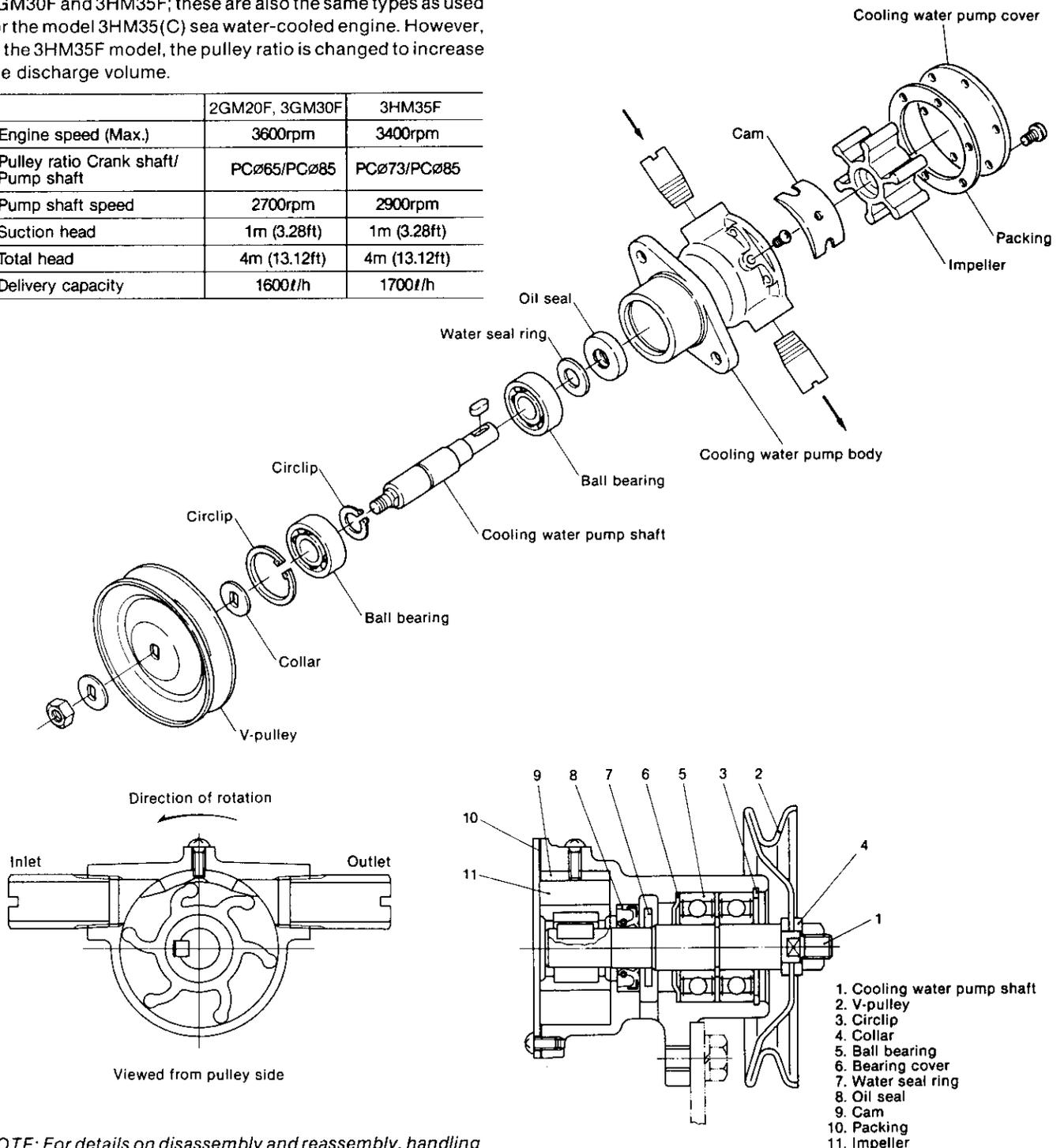
NOTE: For details on disassembly and reassembly, handling precautions and inspection, refer to "Chapter 7, Section 2. Water pump (P.7-5)".
