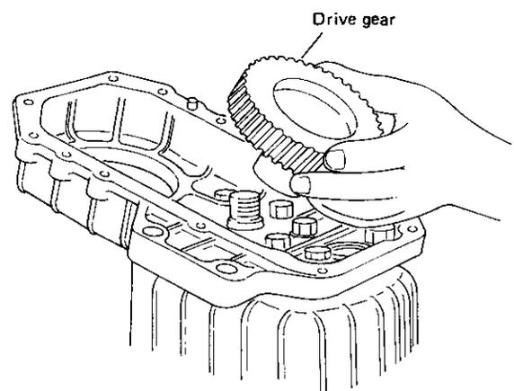
8-11 Remove the V-drive case A fixing bolts, and remove the V-drive case A.
