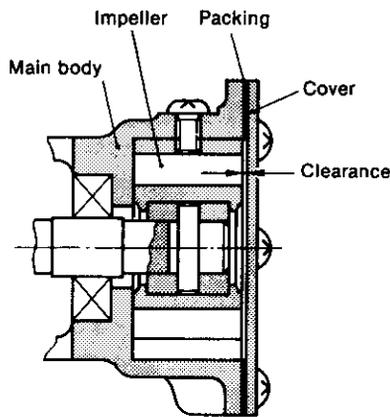
(3) Water pump impeller shaft oil seal section wear.
