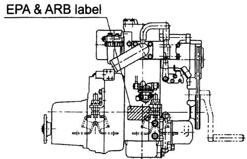
**\*2GM20(C)(V), 2GM20F(C)(V) series:** attached to the intake air silencer side of the rocker arm cover.
