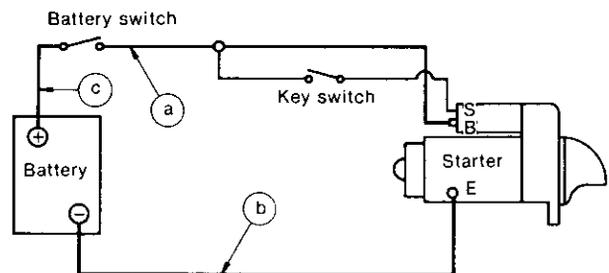
The overall lengths of the wiring between the battery (+) terminal and the starter (B) terminal, and between the battery (-) terminal and the starter (E) terminal should be based on the following table.
