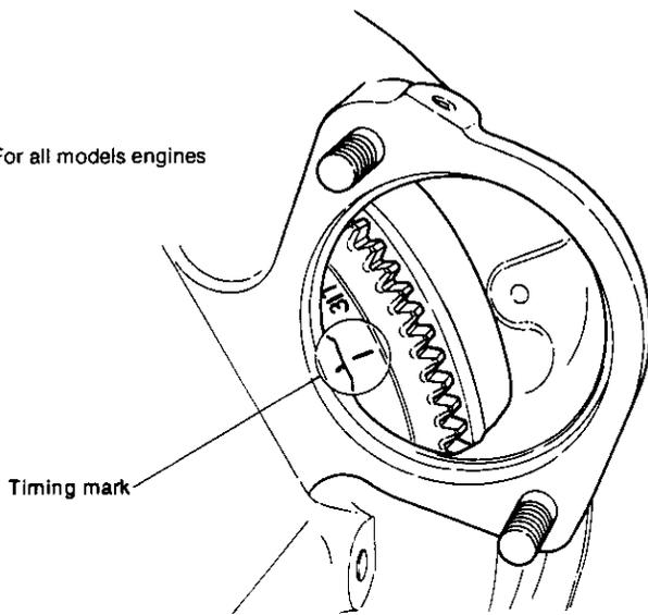
A mark is also punched on the clutch housing for models of 1GM10(C), 2GM20(F)(C) and 3GM30(F)(C)
