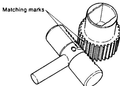
**NOTE:** After attaching the fuel control pinion to the main unit, check its meshing by moving the fuel control rack.
