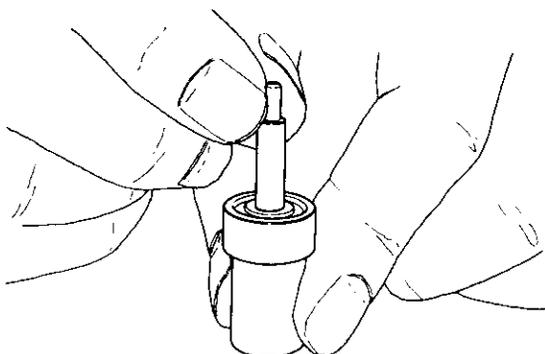
(4) The nozzle must be fitted on the nozzle holder with the nozzle spring retainer loosened.
