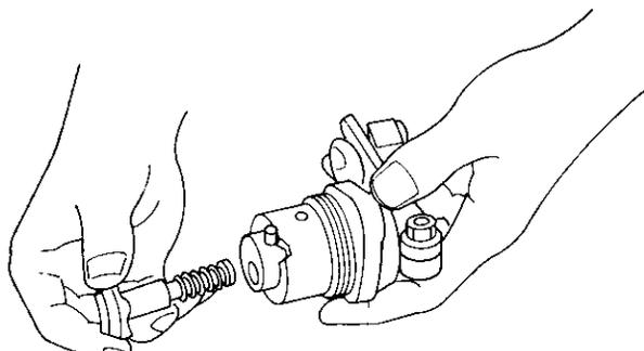
(4) Remove the shift lever to the anti-shift lever side.
