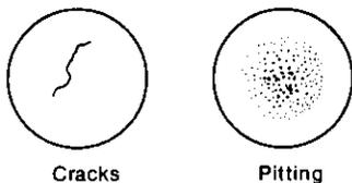
Also, there may be perforated pittings or cracks on the contact surface of the tappet. In such cases, discover the reason for abnormality and replace the tappet.
