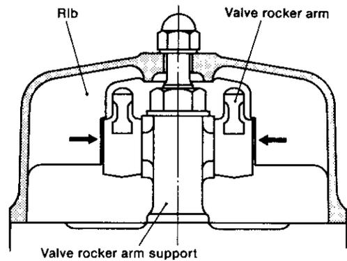
**NOTE:** Take care that the valve rocker arms do not get detached from the valve rocker arm shaft when dismantling or assembling. Replace the bonnet carefully when assembling.
