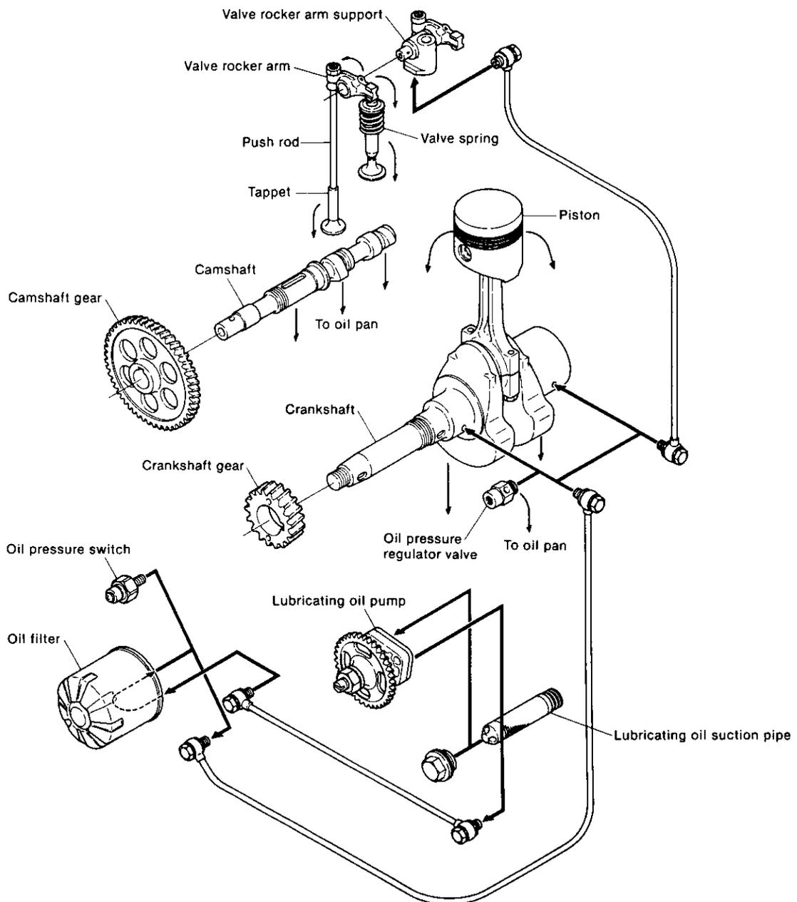
1-2 Lubrication oil passage of model 2GM20(F)(C)
