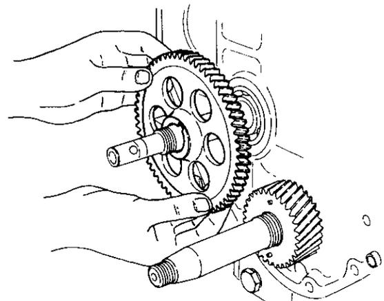
(3) Tighten the camshaft end nut.
