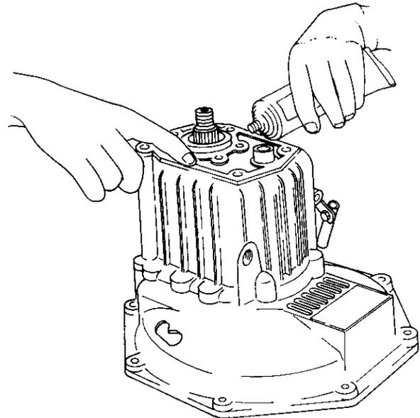
*NOTE: Apply a non-drying type liquid packing to the matching surfaces of the case A and the clutch case.*
