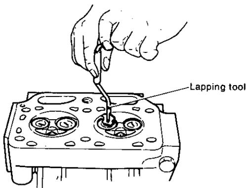
(2) Correcting valve seat width.
