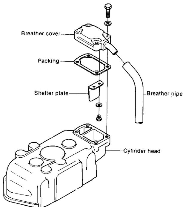
The deflector panel fitted to the breather lid enters the air chamber, and forces air circulation.
