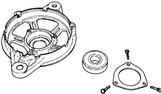
(4) Remove the nut, the brush-holder, and diode fixing nut at the BAT, and the terminal screws of the rear cover. Separate the rear cover from the stator (with the diode and brush holder).
