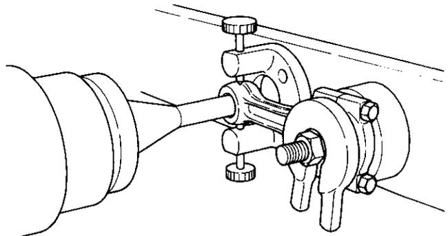
**NOTE:** Attach the bushing to the piston pin so that the pin, coated with engine oil can be pushed into position with your thumb.
