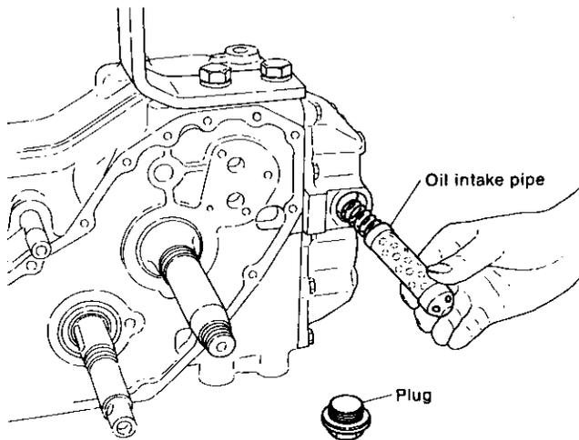
**5-2.7 Install the engine bottom cover (oil pan)**
