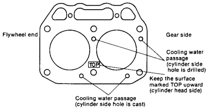
(3) Installing the cylinder head ass'y.
