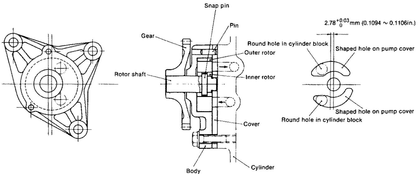
2-1.3 Specifications of lubrication oil pump
