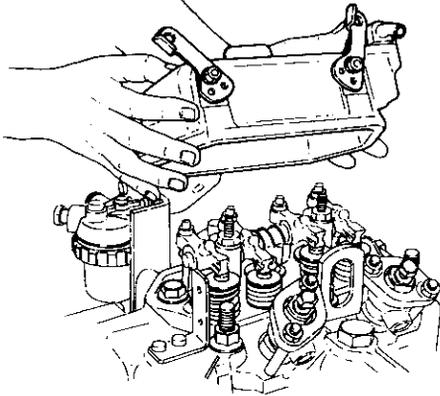
**4-3.13 Remove the exhaust manifold [only for model 3GM30(C)] and the mixing elbow**
