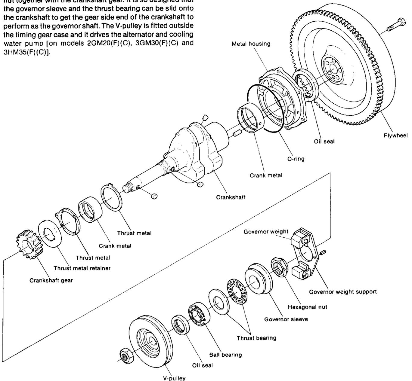
5-1.2 Construction of models 2GM20(F)(C), 3GM30(F)(C) and 3HM35(F)(C) crankshaft assembly
