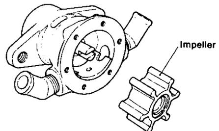
(2) Rubber impeller side wear
