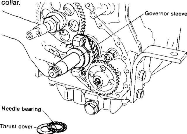
**5-2.18 Install the timing gear case**
