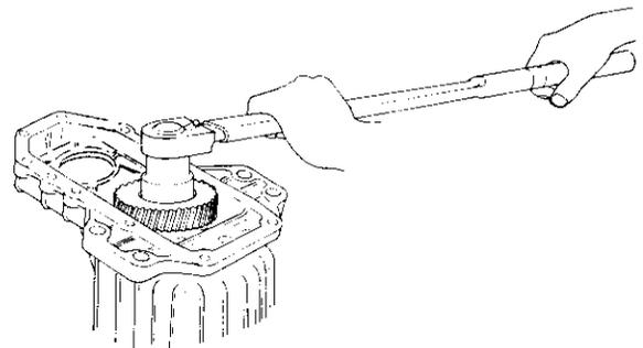
NOTE: Note that the end nut has a left-handed thread.
