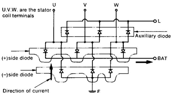
Electric current flows only in one direction in the diode as shown on the previous page. By testing the continuity between terminals (e.g. BAT and U) with the continuity tester, (as shown in the picture), the diode is determined as usable when the continuity is "Yes", but is faulty when it "No".
