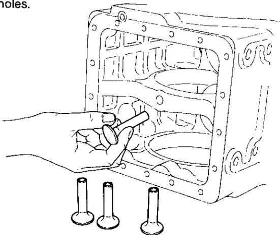
**NOTE:** Assemble the tappets in their original positions, paying careful attention to the cylinder numbers and intake and exhaust groupings.
