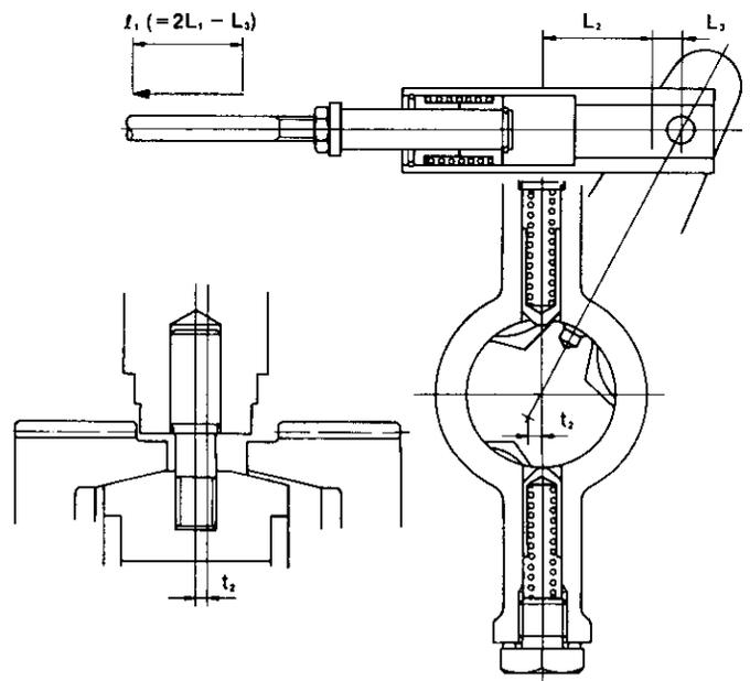
**Position of remote control stroke  $l_1$**
