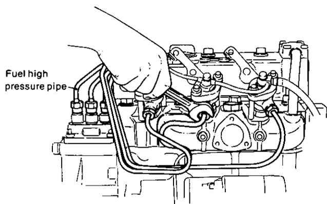
**2-18. Remove the lifting hook at the front of the engine (3GM30, 3HM35)**
