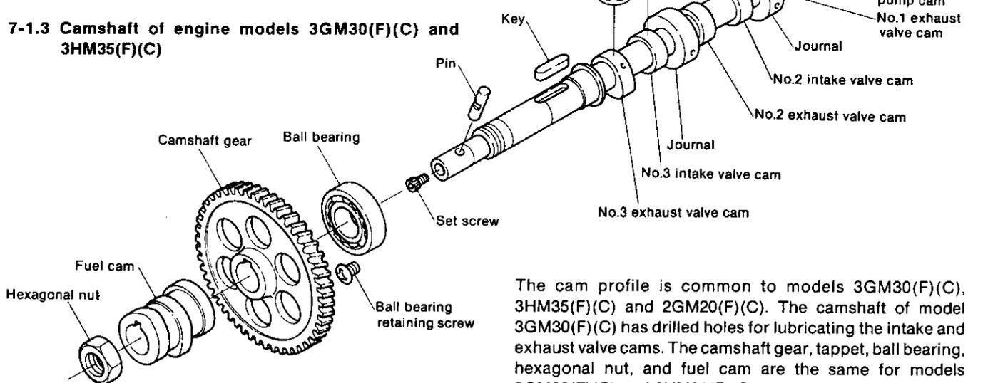
The cam profile is common to models 3GM30(F)(C), 3HM35(F)(C) and 2GM20(F)(C). The camshaft of model 3GM30(F)(C) has drilled holes for lubricating the intake and exhaust valve cams. The camshaft gear, tappet, ball bearing, hexagonal nut, and fuel cam are the same for models 3GM30(F)(C) and 3HM35(F)(C).
