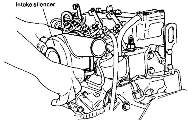
**NOTE:** The intake silencer is the same for both the fresh water and sea water-cooled engines.
