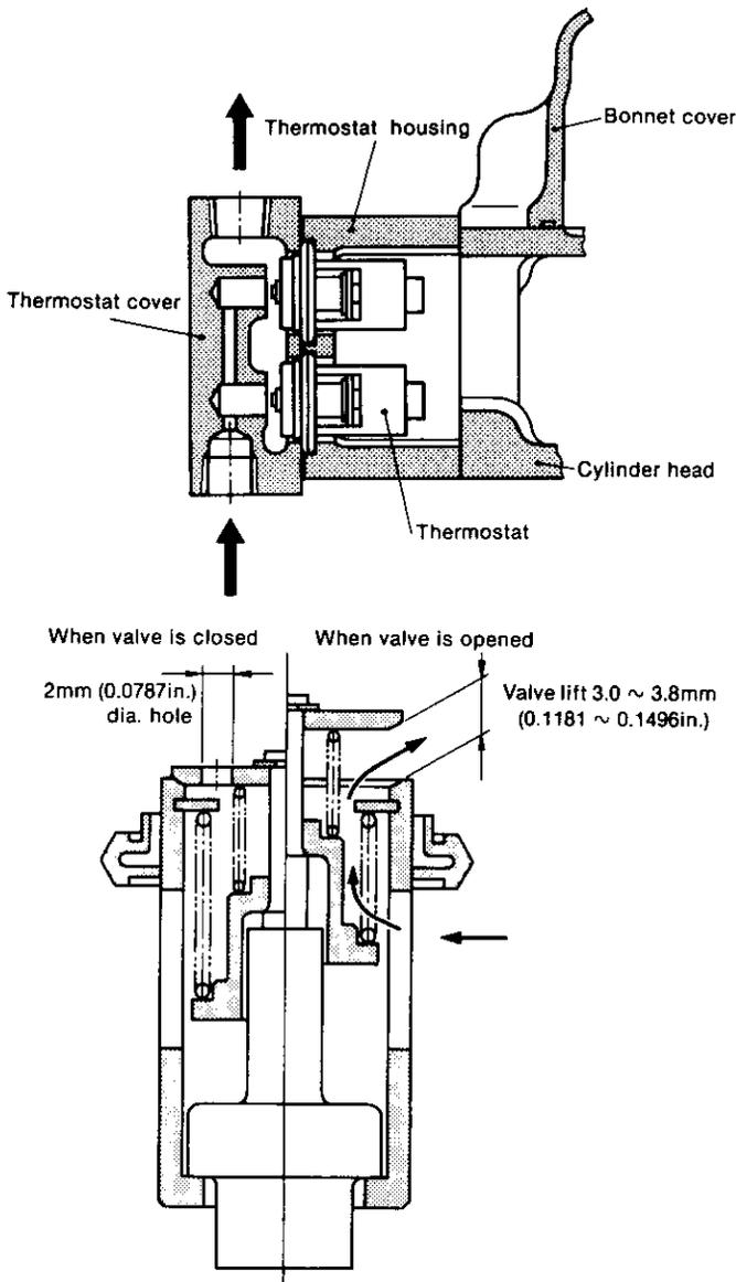
A wax-pellet type thermostat is used for this engine. The "wax-pellet" type is the description given to a quantity of wax in the shape of a small pellet. When the temperature of the cooling water rises, the wax melts and its volume expands. The valve is opened or closed by this variation of volume.
