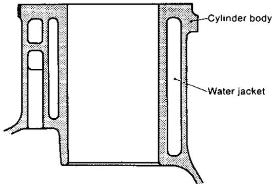
The cylinder block is a high-quality cast iron casting, with integral cylinders and deep skirt crankcase construction. As a result of stress analyses, the shape and thickness of each part has been optimized, and special ribs employed which not only increase the strength and rigidity of the block, but also reduce noise.
