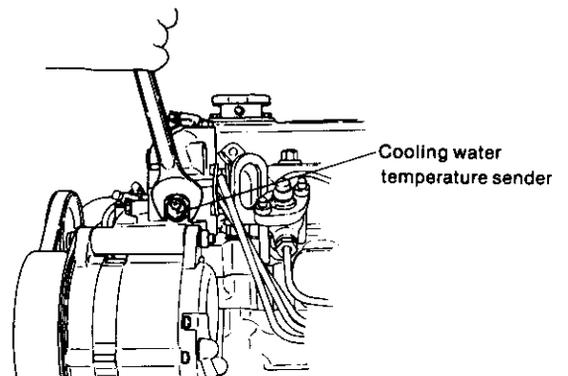
**NOTE:** Apply Threabond No.4 to the threads.
