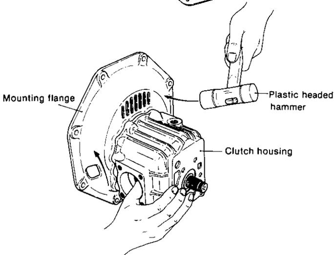
(8) Withdraw the output shaft assembly.
