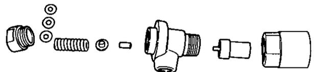
(2) Parts for No.1 cylinder and No.2 cylinder must be kept separate. The nozzle body and nozzle must always be handled as a pair.
