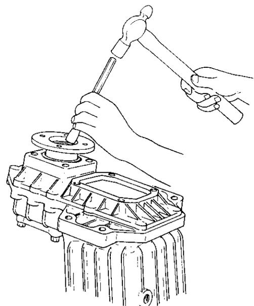
8-7 Remove the end nut, output shaft coupling, and O-ring.
