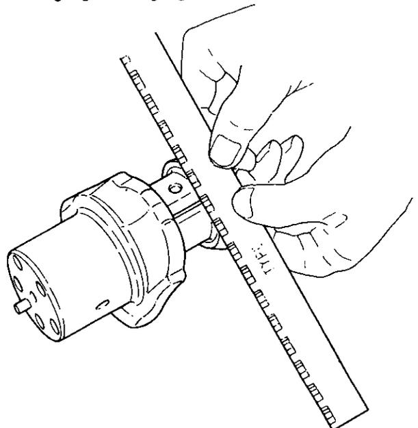
**NOTE:** Never adjust by shims or machine the crank pin bushing. Always replace the crank pin bushing with a new one.
