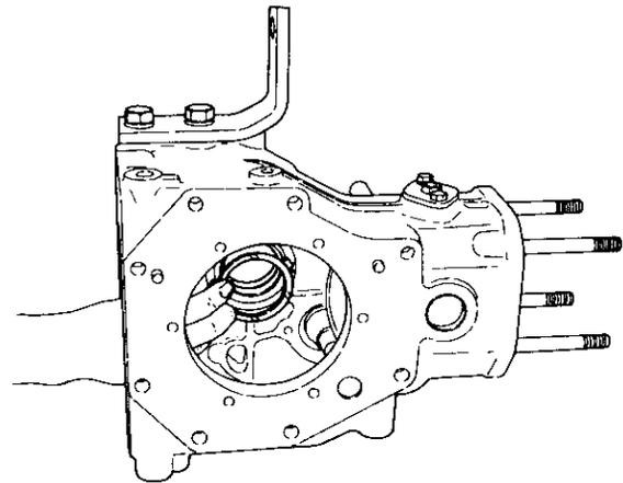
**CAUTION:** Install so that the thrust metal oil groove is at the crankcase side, being careful not to damage the tab.
