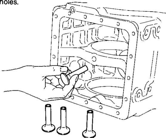
**NOTE:** Assemble the tappets in their original positions, paying careful attention to the cylinder numbers and intake and exhaust groupings.
