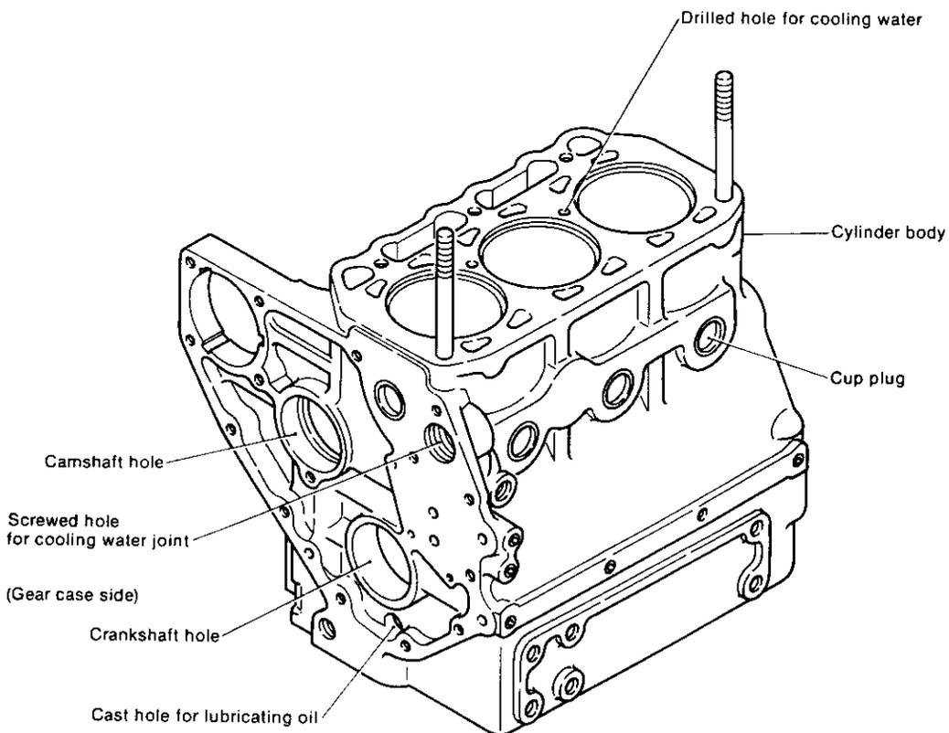
1-1.4 Cylinder of model 3HM35(F)(C) engine
