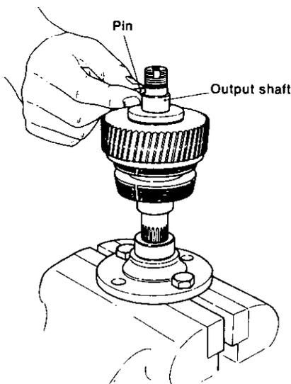
(4) While gripping the drive cone, tap the end of the shaft with a plastic headed hammer, and withdraw the thrust collar B and inner needle bearing race. A pulley extractor may be used.
