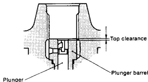
**NOTE:** By inverting and standing the main unit of the pump upright attach the plunger to it carefully.
