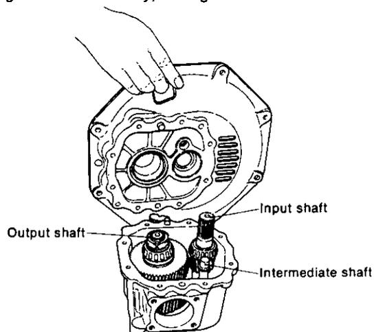
NOTE: Apply non-drying liquid packing to either the mounting flange or the case body.
