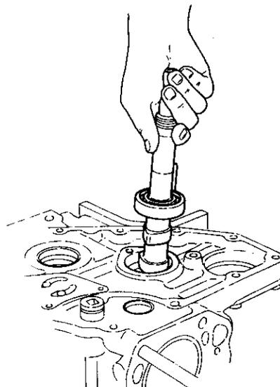
(3) Check that all the tappets are separated from the cam, and pull the camshaft out.
