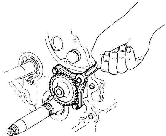
**NOTE:** Do not separate the lubricating pump gear from the rotor shaft. If removed, it cannot be used again. When any part is unusable, replace it as a complete assembly.
