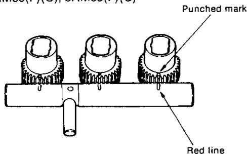
**NOTE:** After attaching the fuel control pinion to the main unit, check its meshing by moving the fuel control rack.
