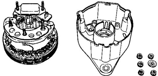
(6) Unsolder the lead wire connection and remove the diode assembly together with the regulator assembly.
