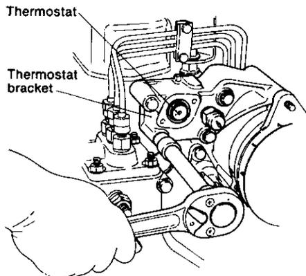
**2-14. Remove the cooling water by-pass connection**
