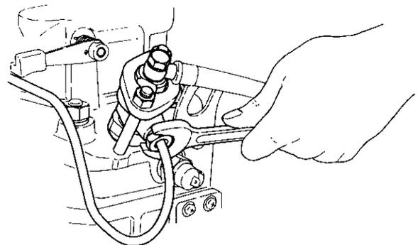
Loosen the nipple on the fuel injection valve side, set the regulator handle to the operating position and the decompression lever to the decompression position, and crank the engine. When no more bubbles appear in the fuel flowing from the end of the injection pipe, retighten the nipple.
