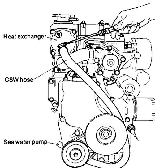
**3-16. Assemble the mixing elbow**
