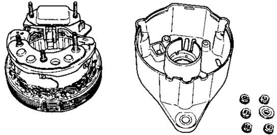
(5) Disconnect the soldered joint of the stator lead wire, and remove the diode and brush regulator assemblies from the stator at the same time.
