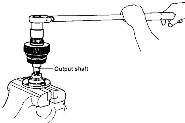
(3) Place the pulley extractor against the end surface of the forward large gear, and withdraw the forward large gear, thrust collar A, cup spring, spring retainer and inner bearing race.
