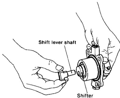
(4) Withdraw the shift lever shaft.
