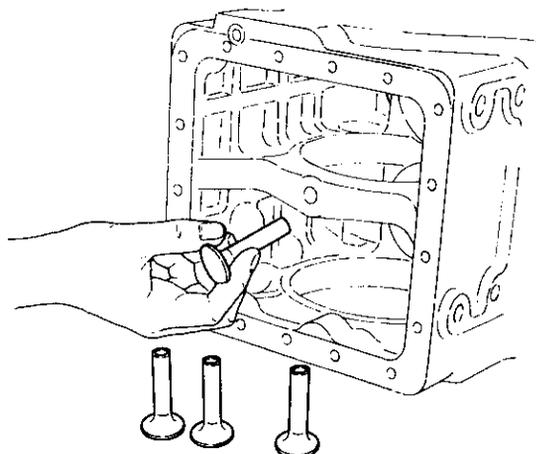
**NOTE:** Arrange the removed tappets by cylinder no. and intake and exhaust groups.
