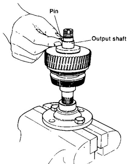
(4) While gripping the drive cone, tap the end of the shaft with a plastic beaded hammer, and withdraw the thrust collar B and inner needle bearing race. A pulley extractor may be used.
