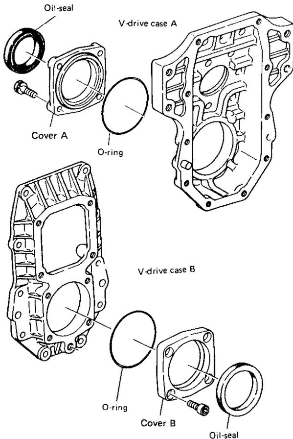
8-14 Remove the bearing outer races from the V-drive cases A and B.
