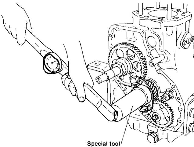
**4-2.25 Remove the camshaft gear**
