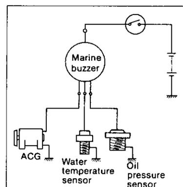
5-6.2 Buzzer for A-type instrument panel
