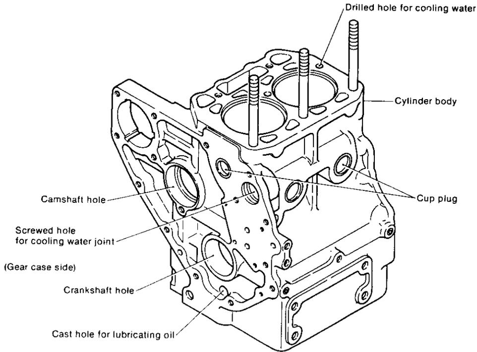
1-1.3 Cylinder of model 3GM30(F)(C) engine
