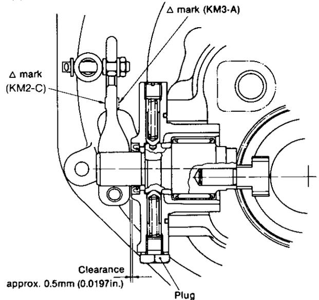
**NOTE:** The clearance between the surface of the side cover and the operation lever is to be 0 ~ 0.5mm (0 ~ 0.0197in.)
