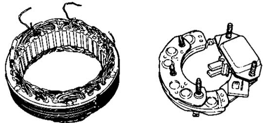
(7) Separate the diode assembly and the brush regulator assembly by removing the 3mm dia rivet which connects these two parts and then unsolder the L terminal connection.
