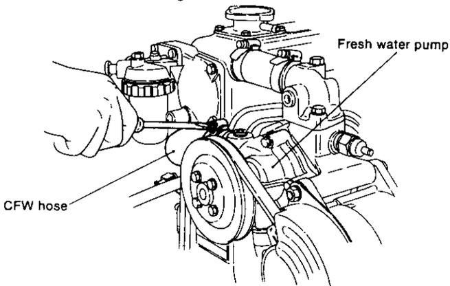
(3) Loosen the hose clamp on the CFW hose between the cylinder head and heat exchanger. The hose clamp at the heat exchanger side or the cooling water outlet connection side only need be loosened.
