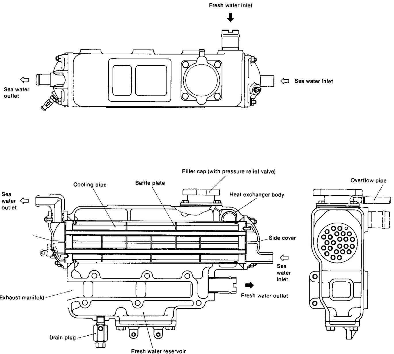
**4-2. Water flow in water cooling tube**
