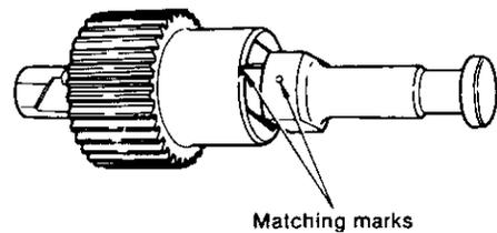
**NOTE:** Invert and stand the main unit of the pump upright and attach the plunger to it carefully.
