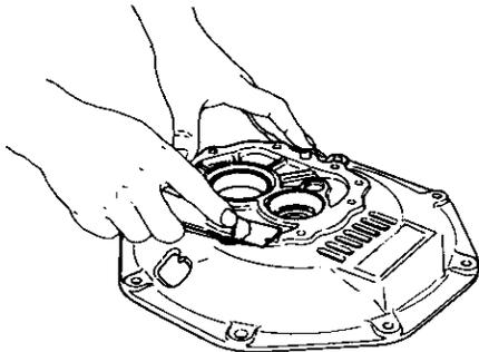
(8) Insert the input shaft and output shaft into the shaft holes of the mounting flange, assemble the mounting flange on the case body, and tighten the bolt.
