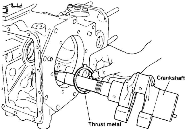
5-2.4 Install the main bearing housing
