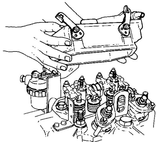
(2) Install the breather pipe to the air intake pipe [intake manifold ... 3GM30(C).]
