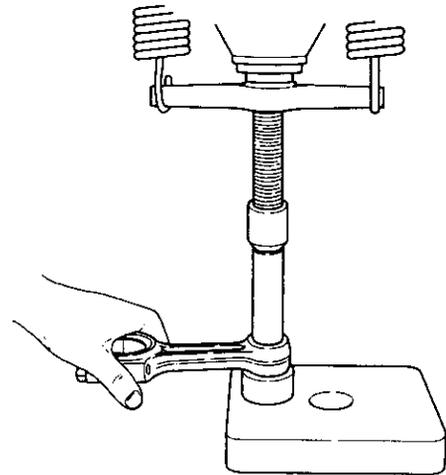
**NOTE:** Force the piston pin bushing into position so that its oil hole coincides with the hole on the small end of the connecting rod.
