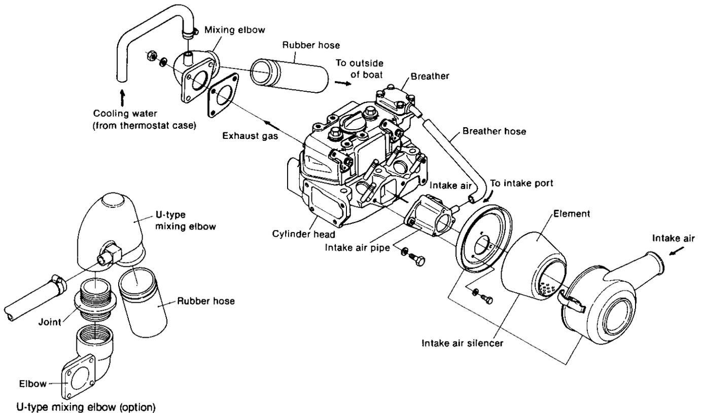
1-3 Intake and exhaust system of models 3GM30(F)(C) and 3HM35(F)(C)
