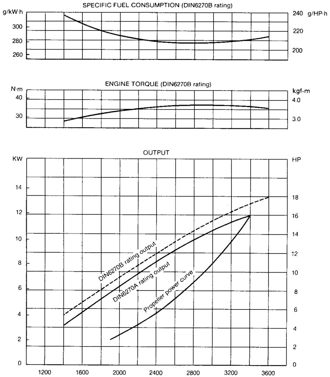
SPEED OF CRANKSHAFT: rpm
