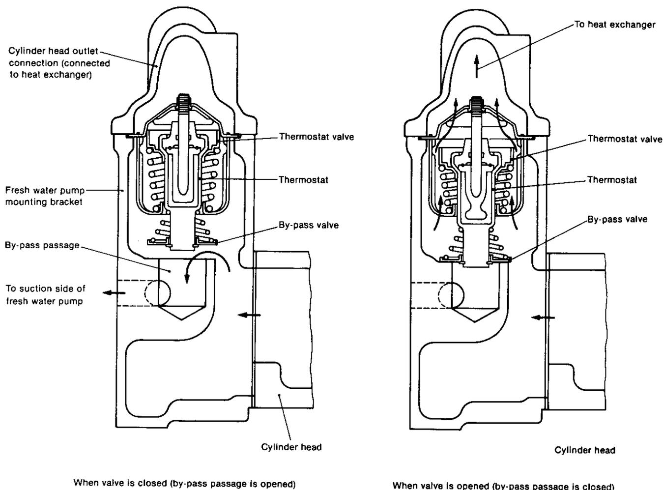
The thermostat opens and closes the by-pass valve and thermostat valve according to the temperature changes of the fresh water in the engine, adjusts the flow of fresh water to the heat exchanger and keeps the fresh water temperature in the engine at the correct level.
