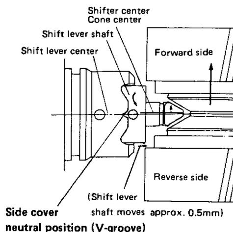
When the location pin of the shift lever shaft falls in the forward position groove of the side cover, (the shift lever shaft moves to the shift lever side approx. 3mm), and the shifter starts to press the drive cone V-groove to the forward large gear side through the spring force.
