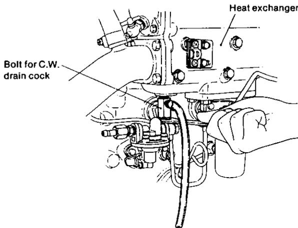
For model 3GMD, connect the pipes after removing the CW drain cock bolt at the bottom of the heat exchanger to prevent the pipe from jamming against the fuel feed pump.
