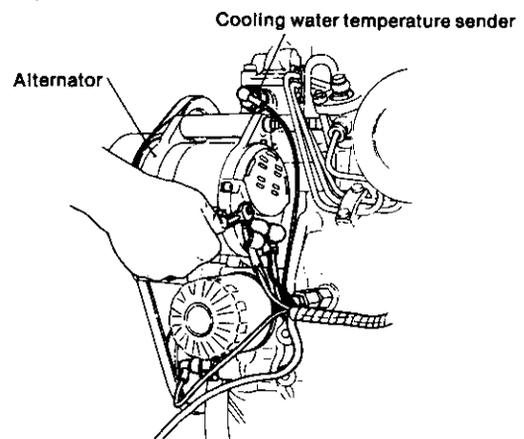
**3-22. Assemble the remote control bracket.**
