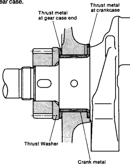
On models 2GM20(F)(C) and 3GM30(F)(C), the value of the side gap is the difference between the width of the basic bearing metal and the width of the journal. The basic bearing for model 2GM20(F)(C) is the intermediate bearing, and for models 3GM30(F)(C) and 3HM35(F)(C) it is the intermediate bearing at the flywheel end.
