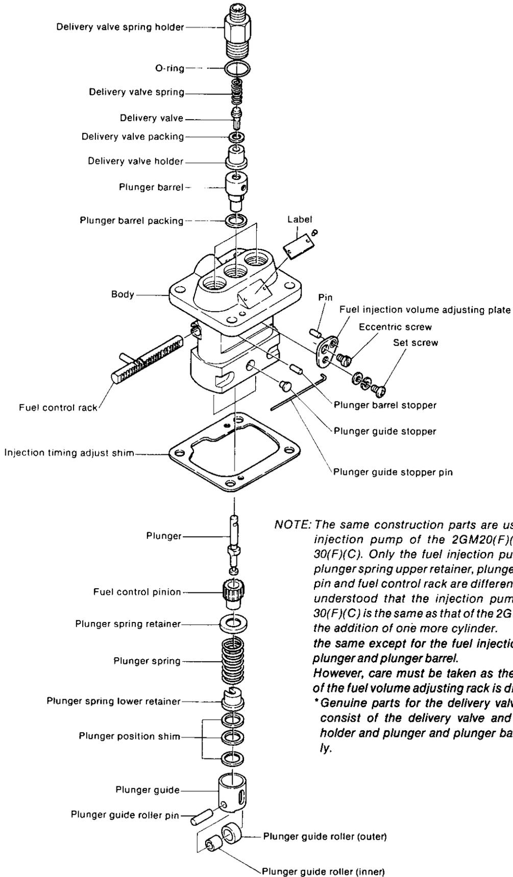
**NOTE:** The same construction parts are used for the fuel injection pump of the 2GM20(F)(C) and 3GM30(F)(C). Only the fuel injection pump body itself, plunger spring upper retainer, plunger guide stopper pin and fuel control rack are different, and it may be understood that the injection pump of the 3GM30(F)(C) is the same as that of the 2GM20(F)(C) with the addition of one more cylinder.
