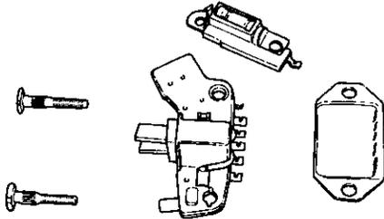
(9) When (1)—(8) above are completed, the alternator is completely disassembled.
