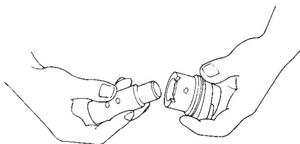
(4) Insert the shifter spring and shifter to the shift lever shaft.
