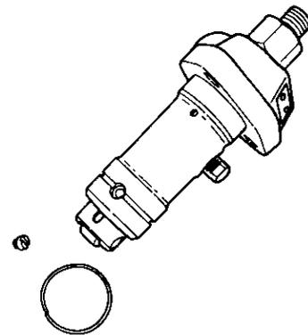
(2) Remove the plunger guide stopper.
