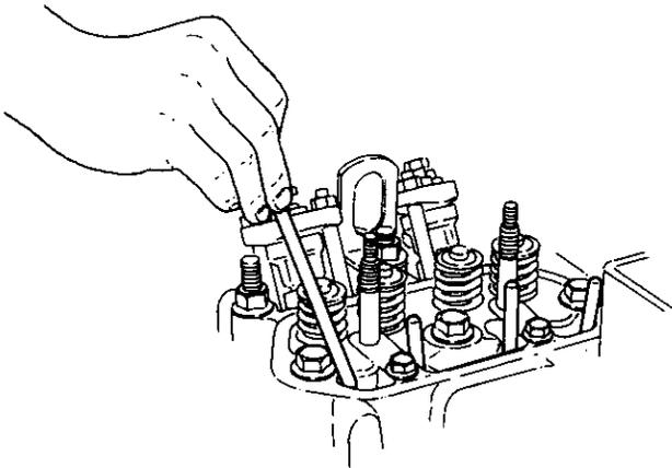
(2) Coat the inside of valve spring retainer with oil
