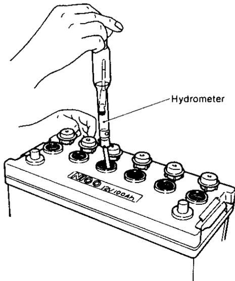
2) Take the specific gravity reading at the top of the scale of the hydrometer.
