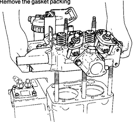
**NOTE:** Clearly identify the front and back of the gasket packing.
