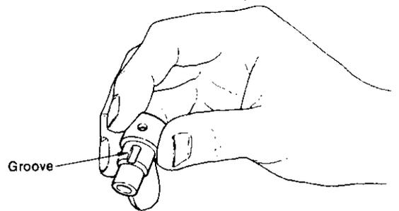
(3) Install the No.1 delivery valve, delivery valve seat and packing.
