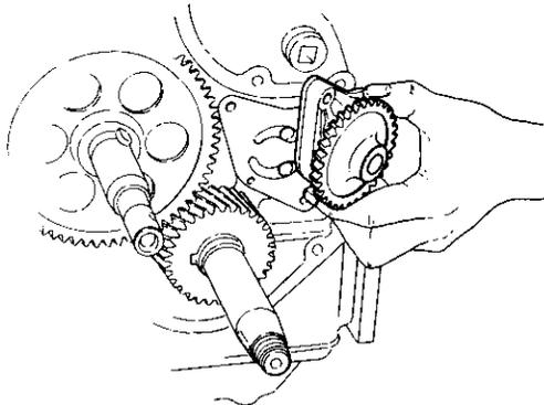
**4-3.27 Remove the camshaft gear and the crankshaft gear**
