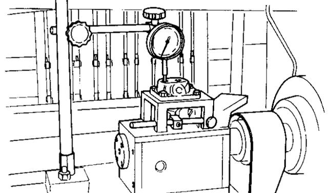
(3) When the plunger top clearance is larger than the prescribed value, remove the plunger guide and insert plunger shims between the plunger spring lower retainer and the plunger guide. Adjust each pump in the same manner.
