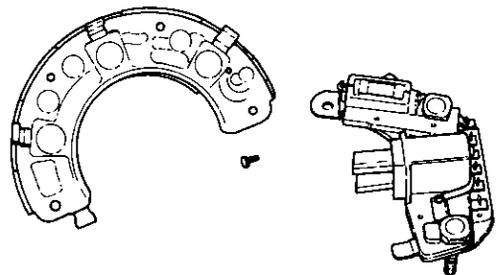
(8) When replacing the IC regulator, it can be removed by unsoldering the regulator's terminals and removing two bolts. Never remove these two bolts except when the regulator is replaced.
