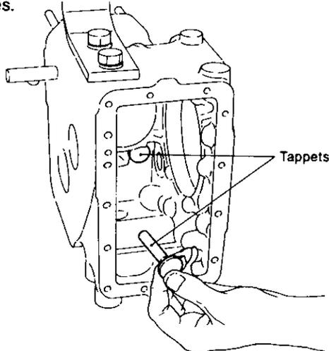
**NOTE:** Assemble the tappets at their original positions, paying careful attention to intake and exhaust.
