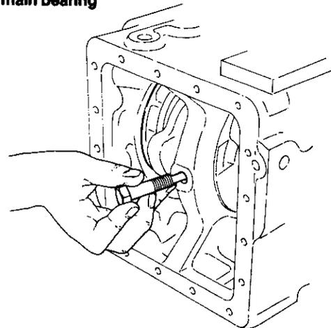
There are two intermediate main bearings, viz. No.1 and No.2, for engine model 3GM30F.
