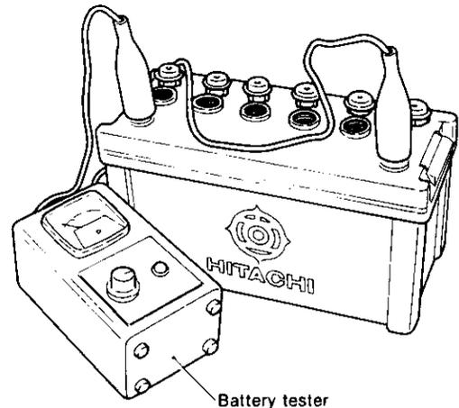
(1) Connect the tester to the battery.
