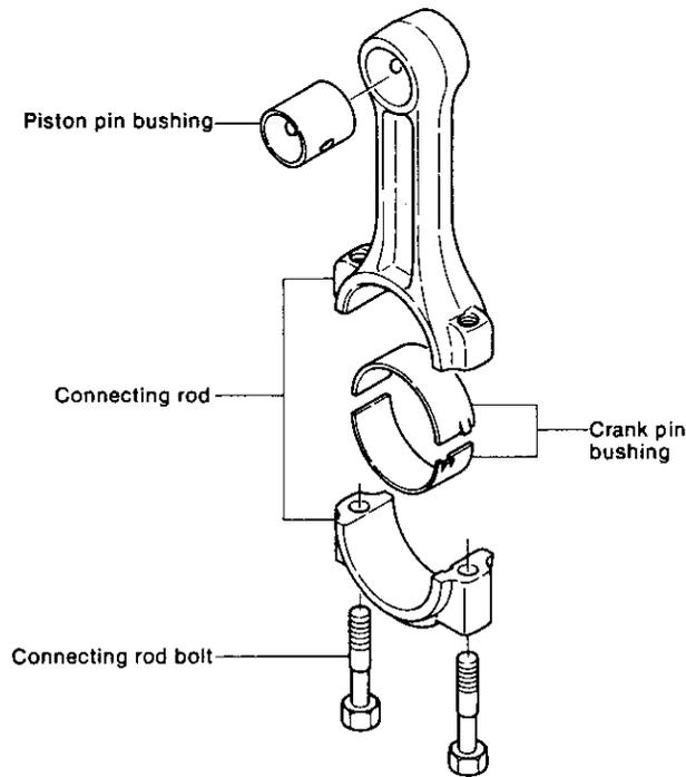
Pass a test bar through the large end and small end holes of the connecting rod, place the bars on a V-block on a stool and center the large end test bar. Then set the sensor of a dial indicator against the small end test bar and measure twist and parallelity. When the measured value exceeds the wear limit, replace the connecting rod. Twisting and poor parallelity will cause uneven contact of the piston and bushing and shifting of the piston rings, resulting in compression leakage.
