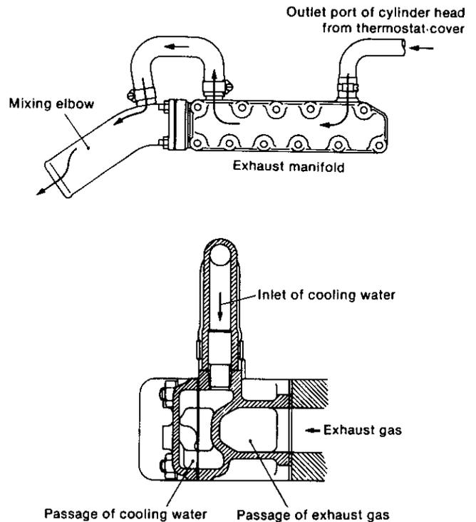
The construction of the exhaust manifold is shown in the figure, and a water chamber is formed between the exhaust manifold and the cover to cool the exhaust gas. The construction of the mixing elbow is the same for models 1GM10(C) and 2GM20(F)(C)
