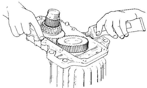
NOTES: 1) Apply a non-drying type liquid packing to the matching surfaces of the V-drive cases A and B.
