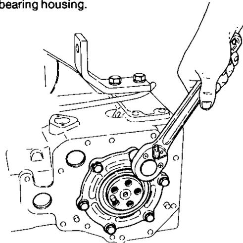
**4-3.32 Remove the mounting bolt of the intermediate main bearing**
