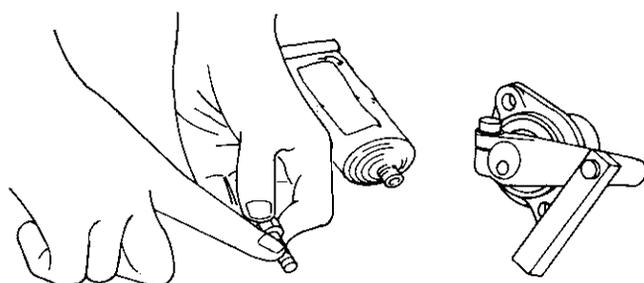
(7) Fit the cable connector to the shift lever.
