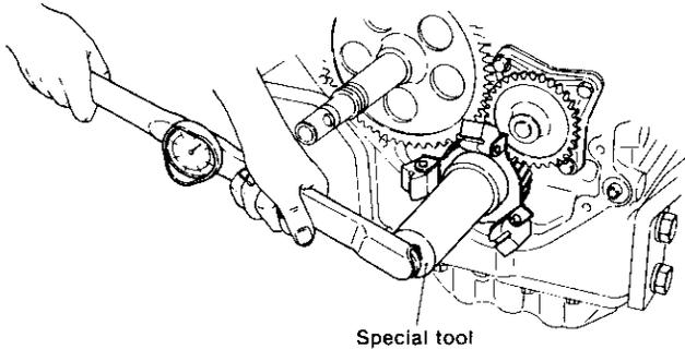
(4) assembling model 1GM10(C) cooling water pump
