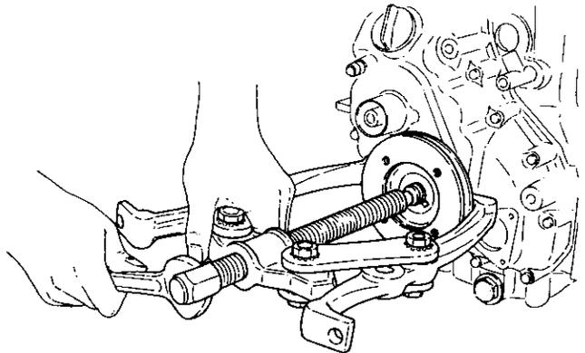
**4-2.17 Remove the injection pump**
