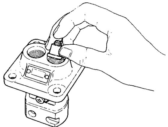
**NOTE:** If the delivery valve tip projects noticeably above the top of the main unit of the pump, the plunger barrel has been installed incorrectly, and must be re-attached.
