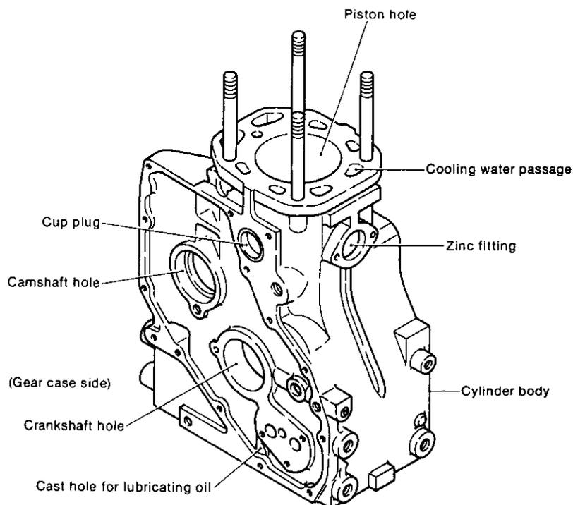
1-1.2 Cylinder of model 2GM20(F)(C) engine
