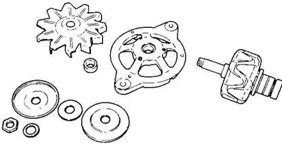
(3) Remove the  $\varnothing 5\text{mm}$  screw from the front cover, and then remove the ball bearing.
