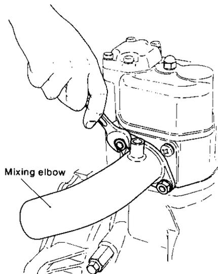
Check for carbon build-up and for corrosion inside the pipe, and repair or replace the pipe if faulty. Also, inspect the mixing elbow mounting threads for cracking and corrosion.
