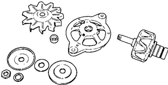
(4) Next, remove the bearing attached to the front cover. Loosen the bearing protector mounting bolts (M4) and pull the bearing by applying pressure to the bearing from the front cover.
