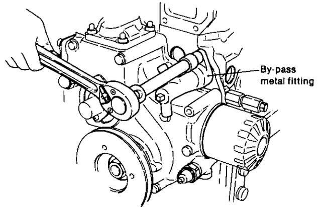
(2) Extract the by-pass connection screwed into the cylinder block.
