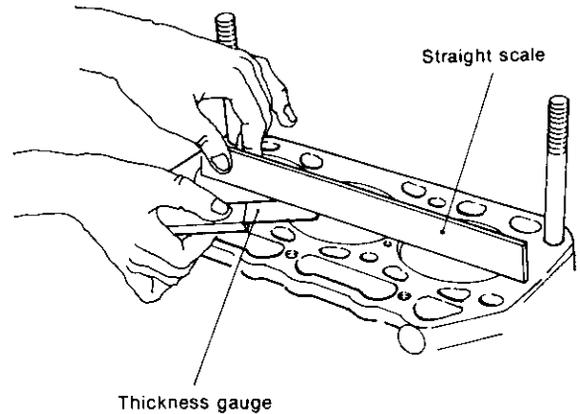
Measurement is to be carried out on the 4 sides and 2 diagonal lines as shown in the figure, and the largest value of clearance for each measurement is to be taken as the amount of distortion.
