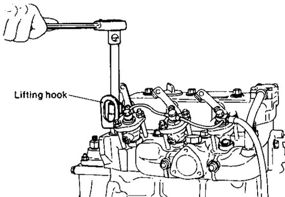
**NOTE:** Use the special lifting hook for the fresh water-cooled engine.
