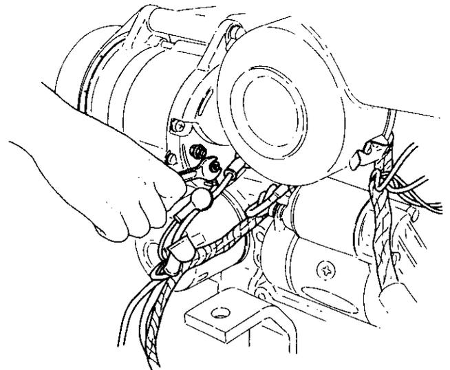
**2-12. Install the remote control cables**
