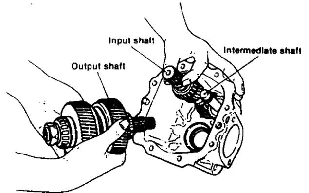
(9) Take out the intermediate shaft and input shaft. When taking out the intermediate shaft, place a bolt or spacer on the shaft hole of the case, and drive the shaft out by tapping it lightly.
