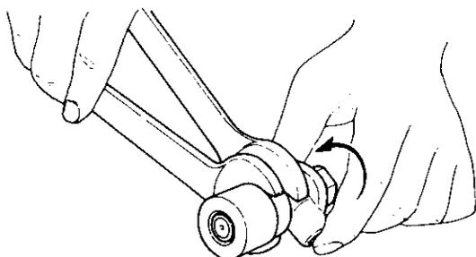
(5) When installing the injection nozzle on the cylinder head, tighten the nozzle holder nuts alternately, being careful to tighten them evenly.
