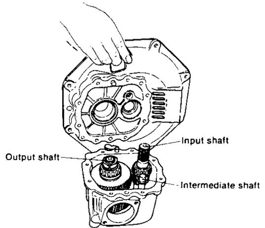
**NOTE:** Apply non-drying liquid packing to either the mounting flange or the case body.
