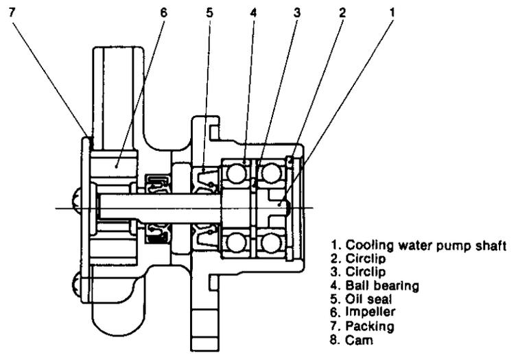
2-1.2 Cooling water pump of engine models 2GM20(C) and 3GM30(C)
