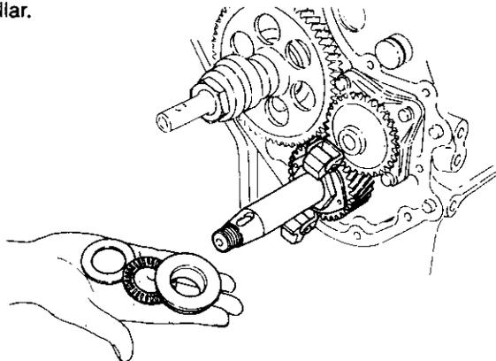
**5-3.17 Install the timing gear case**
