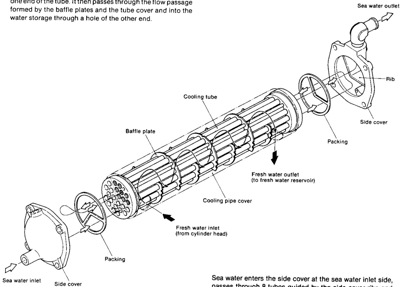
Sea water enters the side cover at the sea water inlet side, passes through 8 tubes guided by the side cover ribs and then leaves the side cover at the sea water outlet side. Here it passes through another 8 tubes guided by the side cover ribs, and returns to the side cover at the inlet side. At the inlet side, it is guided by the remaining 8 tubes as from the outlet side, and then flows out to the mixing elbow from the outlet connection via the side cover at the outlet side.
