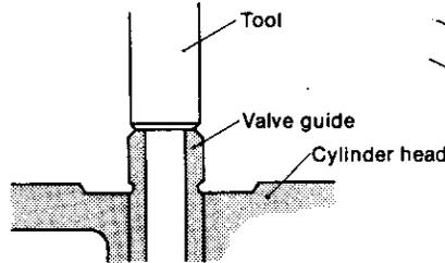
2) Using the above tool, drive the valve guide into position by starting from the valve spring side and finish the inside diameter with a reamer.
