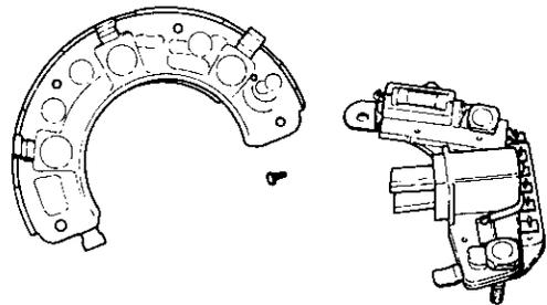
2) To replace the IC regulator, disconnect the soldered joint of the IC regulator and pull out the two bolts. Do not remove these two bolts except when replacing the IC regulator.
