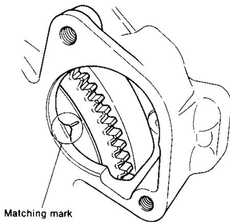
With respect to models 1GM10(C), 2GM20(F)(C) and 3GM30(F)(C) only, a projection which serves as the matching mark is provided in the cast hole of the clutch housing.
