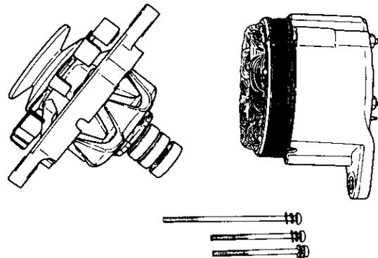
(2) When disassembling the front side pulley and fan, front cover and rotor, clamp the rotor in a vice within copper plates and loosen the pulley nut, as shown in the figure.
