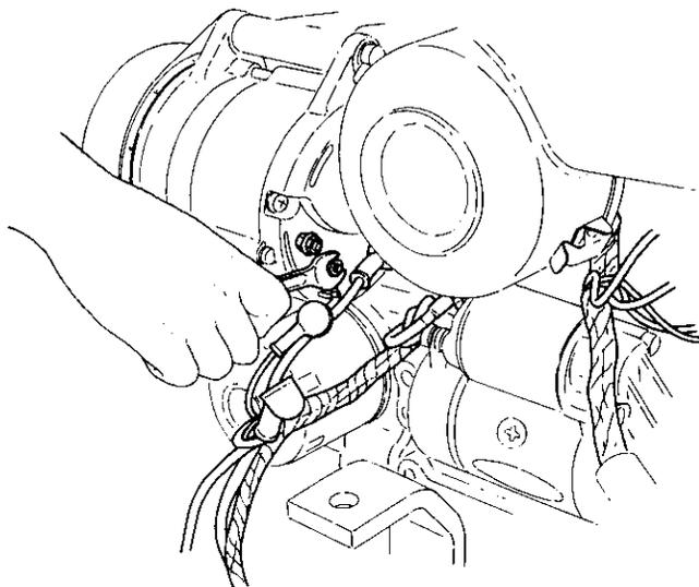
5-3.32 Install the remote control cables
