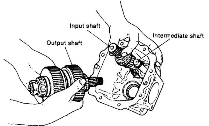
(9) Take out the intermediate shaft and input shaft. When taking out the intermediate shaft, place a bolt or spacer on the shaft hole of the case, and drive the shaft out by tapping it lightly.
