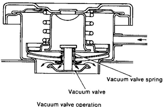
When the cooling system pressure is within the specified range  $0.9\text{kgf/cm}^2$  ( $12.80\text{ lb/in}^2$ ), the pressure valve and vacuum valve are tightly closed on their valve seats. When pressure rises, the pressure valve opens and vapor is discharged from the overflow pipe. When the water cools down and the pressure in the system is lower than atmospheric pressure, the vacuum valve opens and air enters the system through the overflow pipe.
