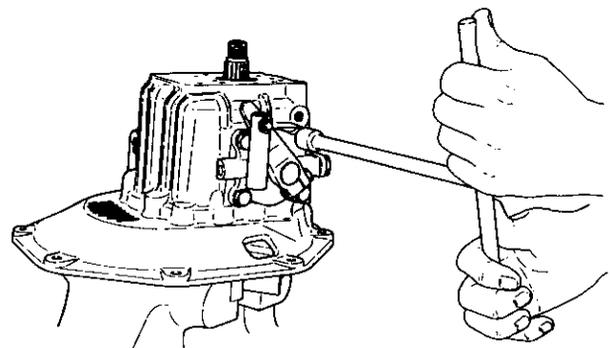
(7) Remove the bolts which secure the mounting flange to the case body, give light taps to the left and right with a plastic headed hammer while supporting the clutch case with your hand, then remove the mounting flange.
