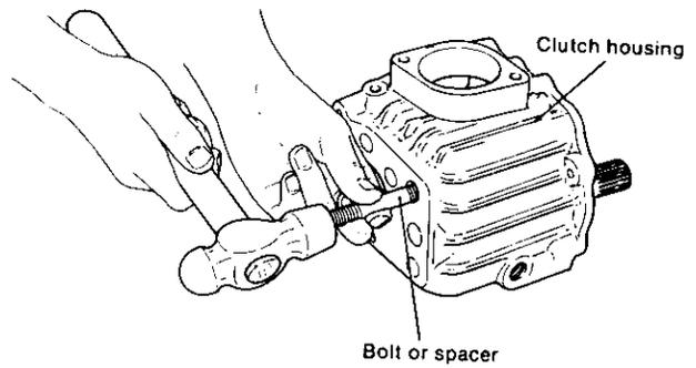
(8) Withdraw the output shaft assembly.
