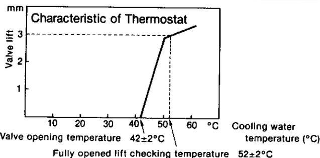
When the seawater temperature is below 42°C, the pumped-up seawater is discharged outside directly from the thermostat section, and circulation of the cooling water into the cylinder is stopped until the water temperature rises. When the water temperature reaches 52°C, the thermostat valve is fully opened.
