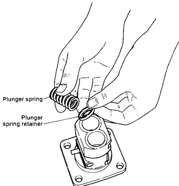
**NOTE:** The plunger spring retainer should face the underside the pump.
