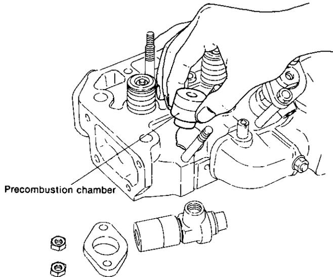
(3) Removing the intake and exhaust valve ass'y
