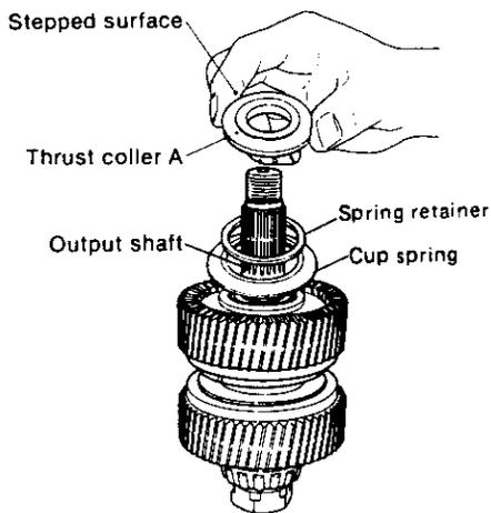
**NOTE:** 1) Fit thrust collar A so that the stepped surface faces the roller bearing side.
