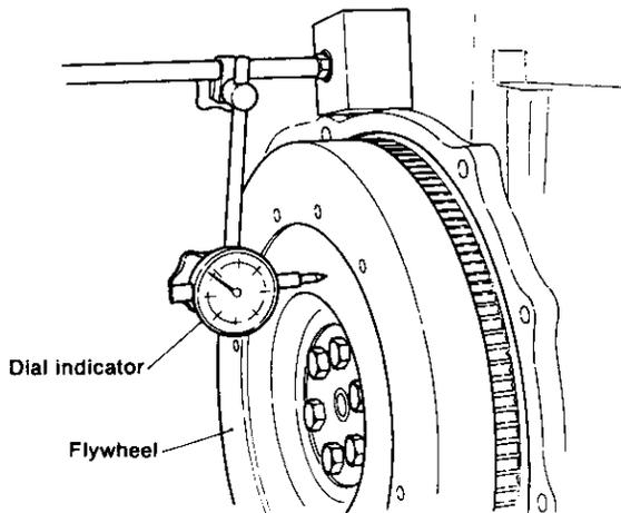
5-3.3 Side gap maintenance standard and wear limit
