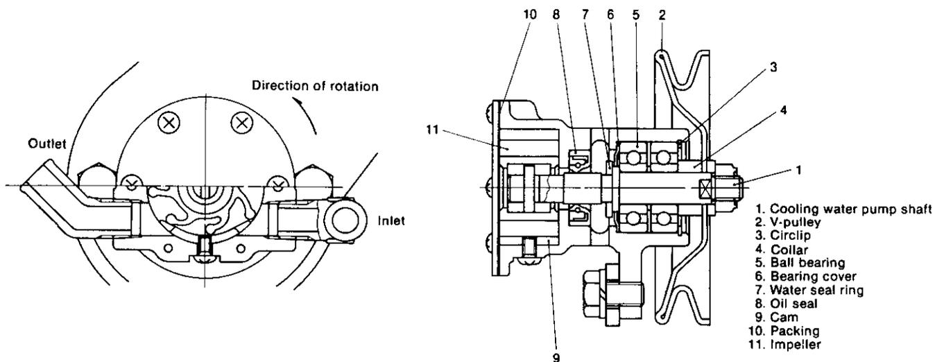
2-1.3 Cooling water pump of engine model 3HM35(C)
