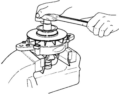
(3) When the fan and pulley have been removed, the rotor can be pulled from the front cover by hand.
