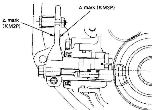
(2) Insert the shift lever shaft to the side cover.
