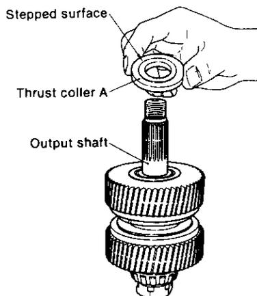
**NOTE:** Fit thrust collar A so that the stepped surface faces the bearing side.
