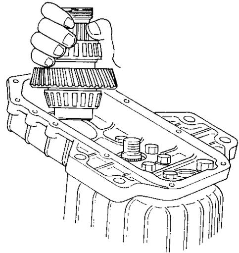
8-10 Remove the end nut, and drive gear from the output shaft.
