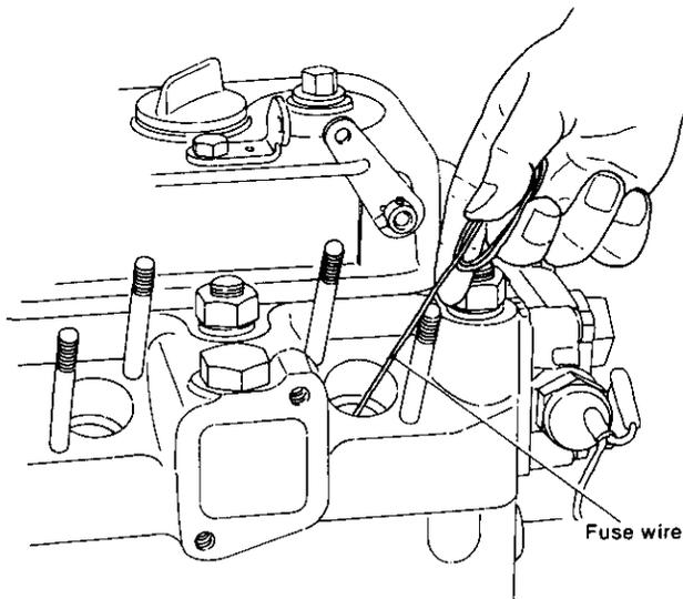
3) Lower the piston at the side to be measured.
