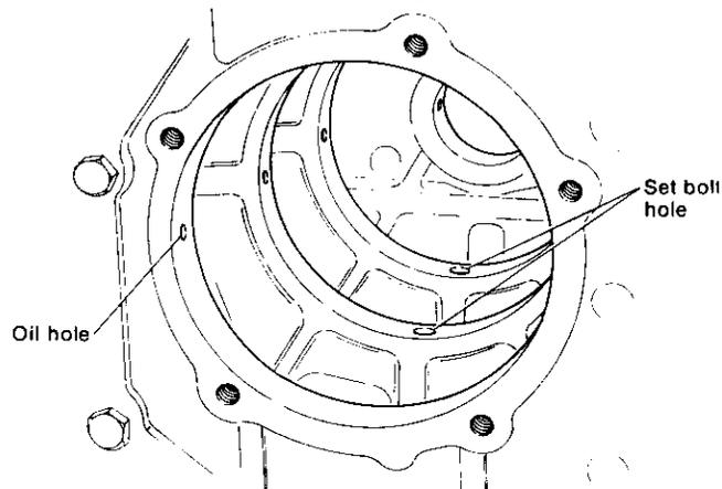
(4) Attaching the intermediate main bearing housing set bolts.
