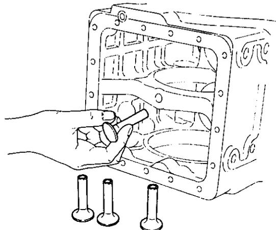
**NOTE:** Arrange the removed tappets by cylinder no. and intake and exhaust groups.
