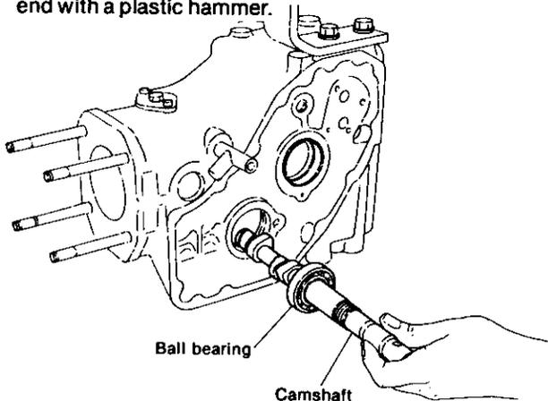
**NOTE:** Be careful not to damage the groove in the end of the shaft.
