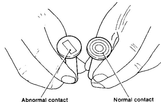
Since the tappet and cam are offset, the tappet rotates in an up and down movement during operation, so there is no uneven contact.
