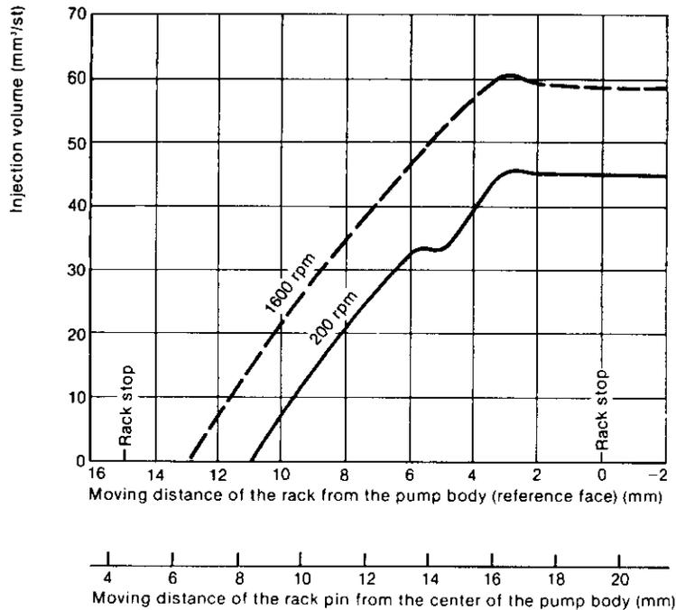
2-3 Operation of fuel injection pump
