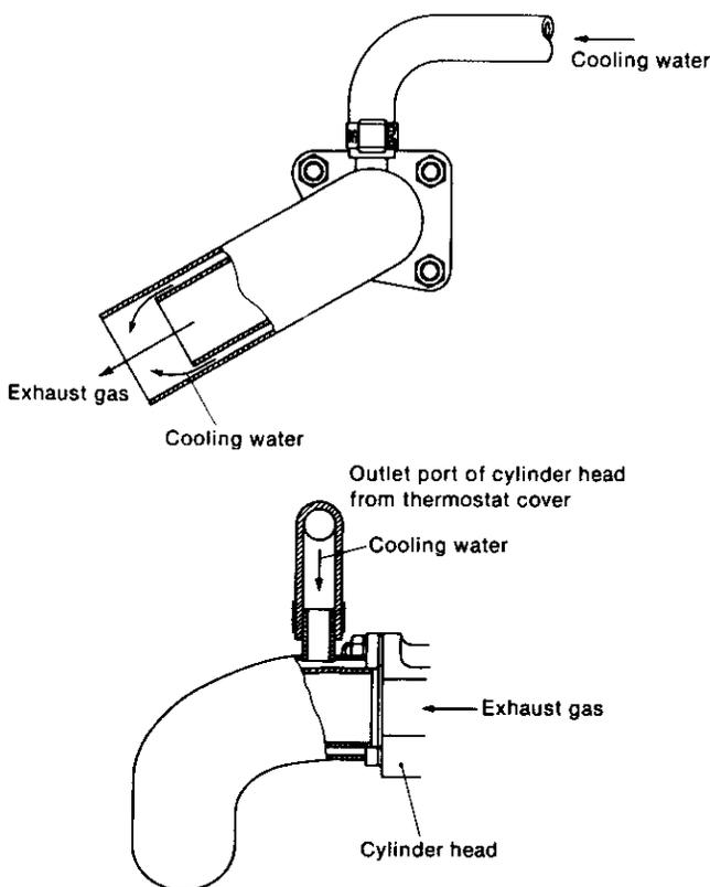
As shown in the figure, the construction for models 1GM10(C) and 2GM20(F)(C) is such that there is no exhaust manifold and the mixing elbow is fitted to the exhaust gas outlet port. A double construction technique has been adopted for the mixing elbow; as the exhaust gas passes through it the cooling water passes round the outside to cool the exhaust gas and then the gas and water mix close to the outlet port.
