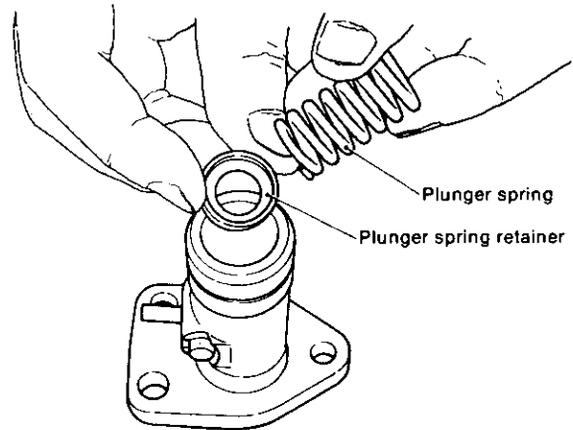
**NOTE:** The plunger spring retainer should face the underside of the pump.
