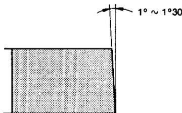
(3) The oil ring is a chrome-plated coil expander having a small contacting face, and exerts high pressure against the cylinder liner wall. Oil splash at the bottom of the sliding face is excellent, and its oil control effect is high.
