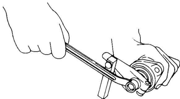
(5) Remove the oil-seal and O-ring.
