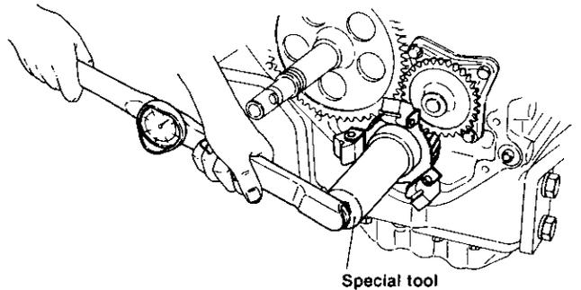
Remove the crankshaft end nut and remove the governor weight assembly.
