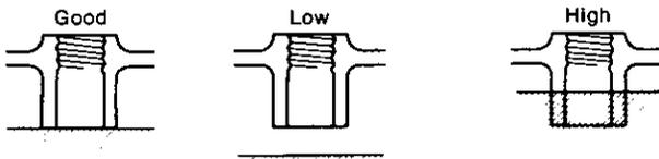
Check the electrolyte level every 7 to 10 days. The electrolyte must always be 10 ~ 20mm over the tops of the plates.
