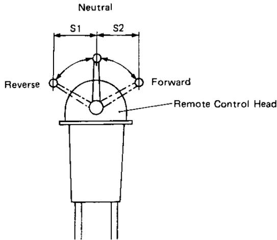
The stroke between the neutral position → forward position (S2), and the neutral position → reverse position (S1) must be equalized.
