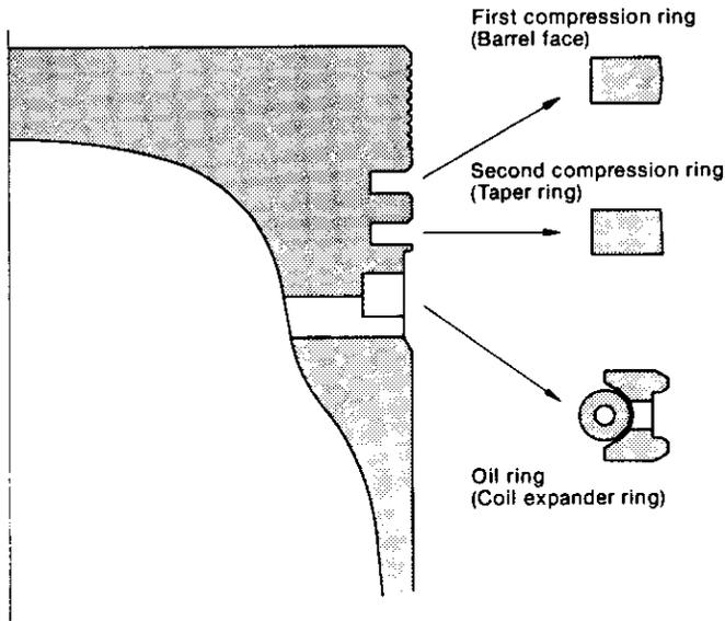
(1) The first compression ring is a barrel face ring that effectively prevents abnormal wear caused by engine loading and combustion gas blowby at initial run-in. The sliding surface is hard chromium plated.
