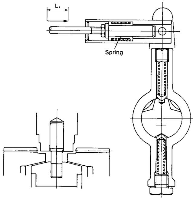
**L<sub>1</sub> position of remote operation stroke**
