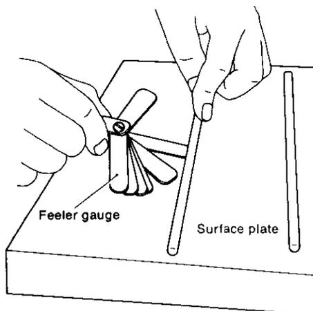
Check both ends for wear and peeling, and replace the push rod if faulty.
