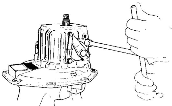
(7) Remove the bolts which secure the mounting flange to the case body, give light taps to the left and right with a plastic headed hammer while supporting the clutch case with your hand, then remove the mounting flange.
