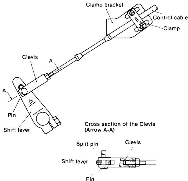
**NOTE:** Since the cable stroke may be insufficient, two holes are drilled in the shift lever.
