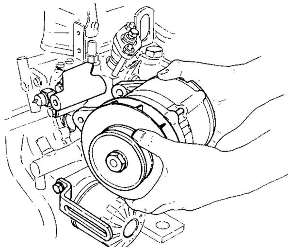
(2) Install the V-belt and tighten the adjusting bolt while adjusting the V-belt tension.
