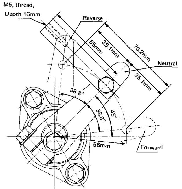
2-5 Adjustment of shifting device
