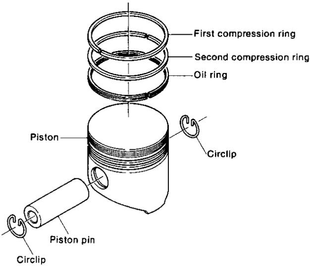
A complete set of piston rings consists of two compression rings and one oil ring.
